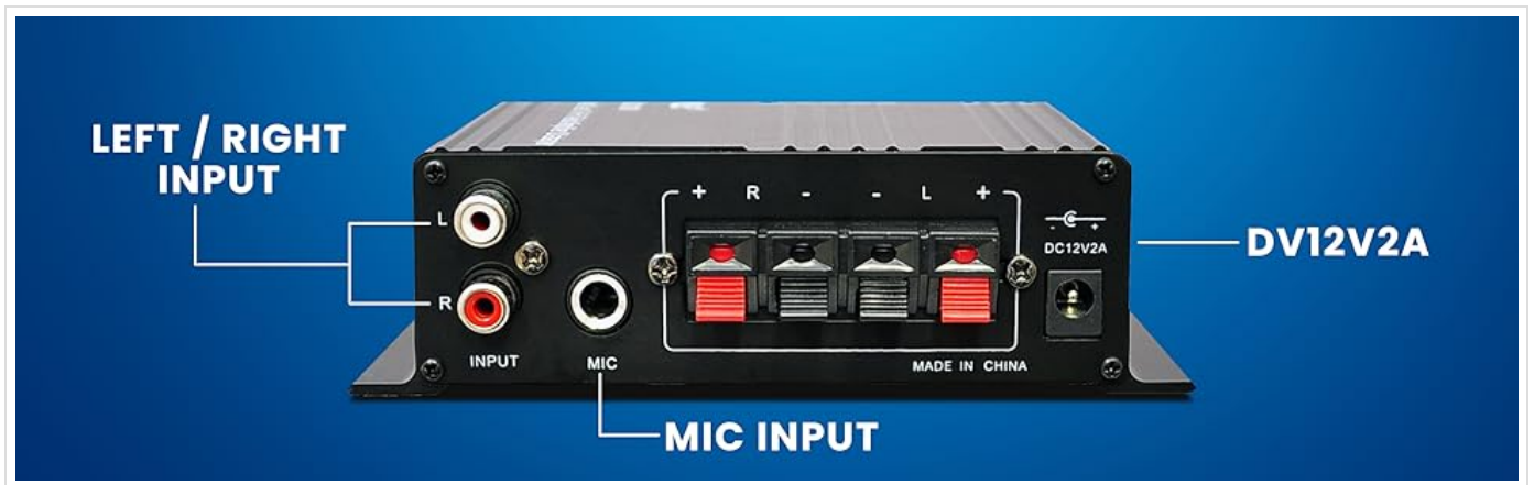
Image 4.4: Close-up view of the PFA200 amplifier's rear panel, highlighting the input and output connections.
