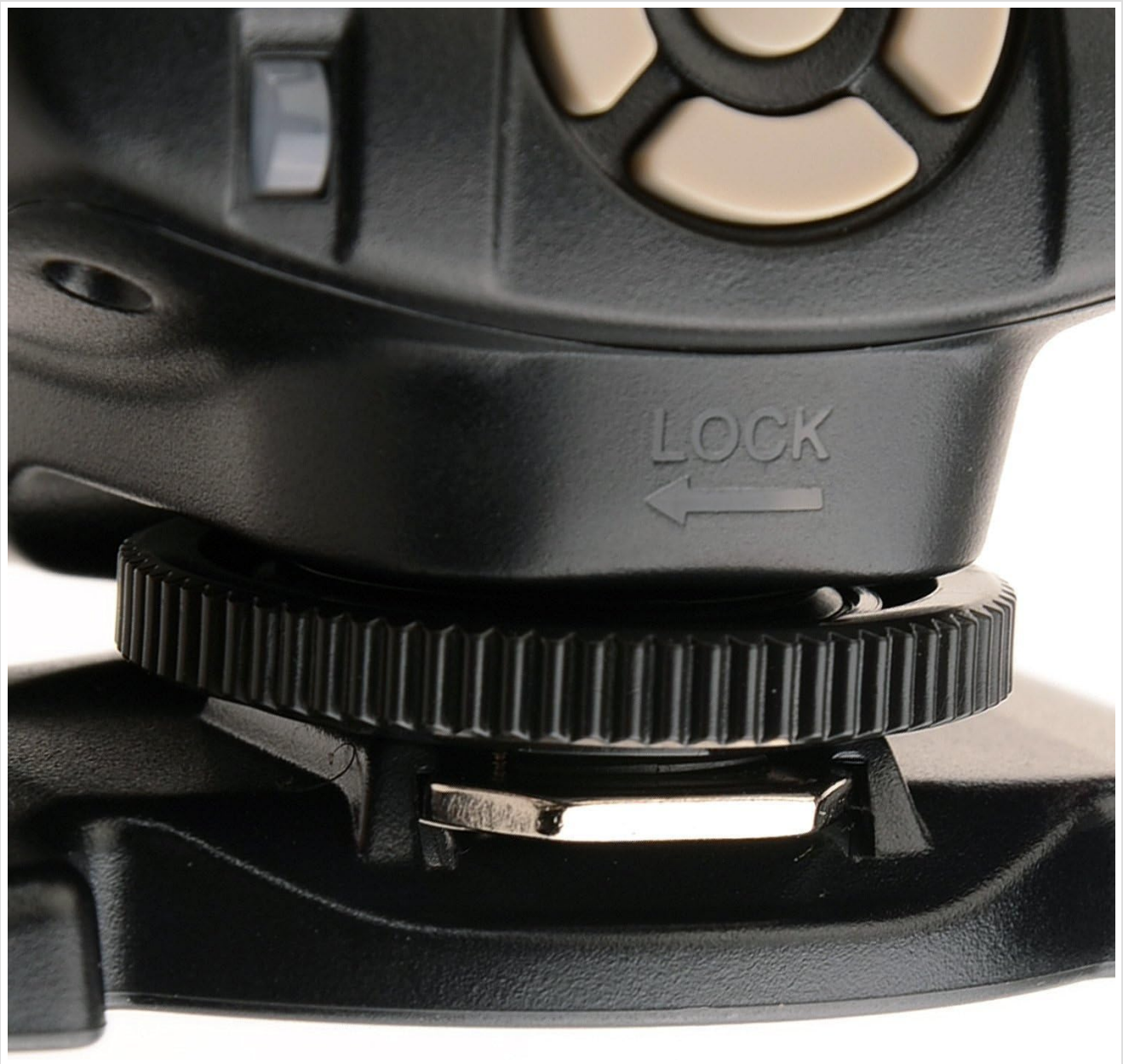
Figure 4.2: YN560-TX PRO N Transmitter, showing its hot shoe mount.
