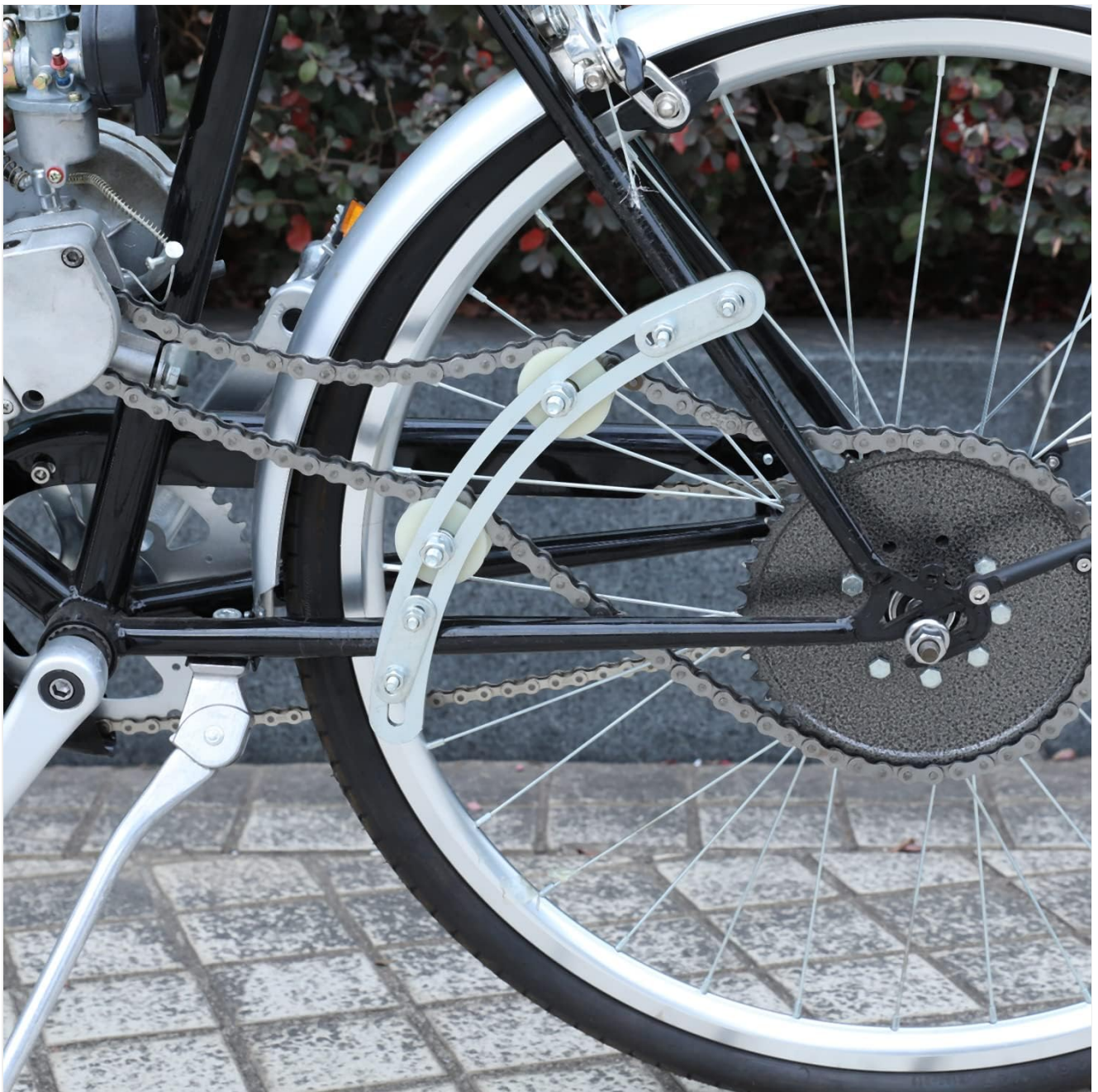
Image 4.2: The chain tensioner installed on a motorized bicycle, showing chain routing.
