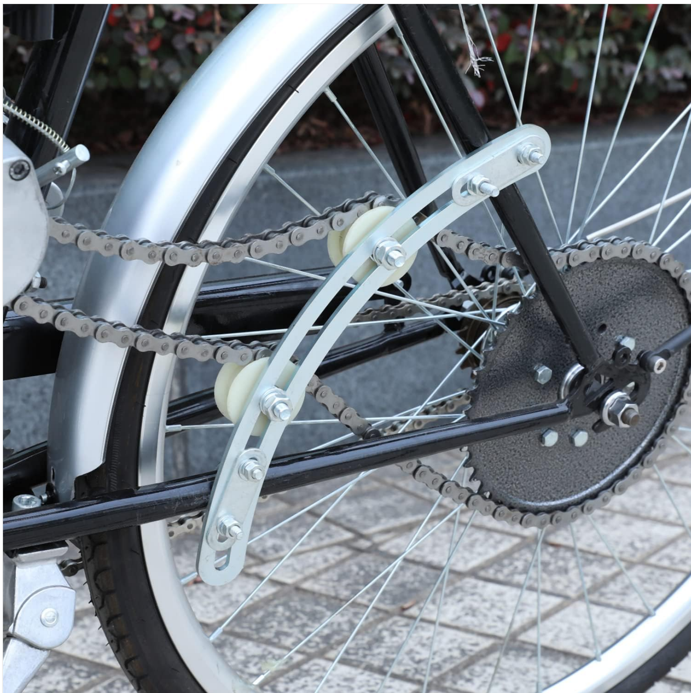
Image 5.1: The chain tensioner actively guiding the chain on a motorized bicycle.
