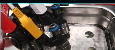
Supports Cleaning of Gasoline Injectors
