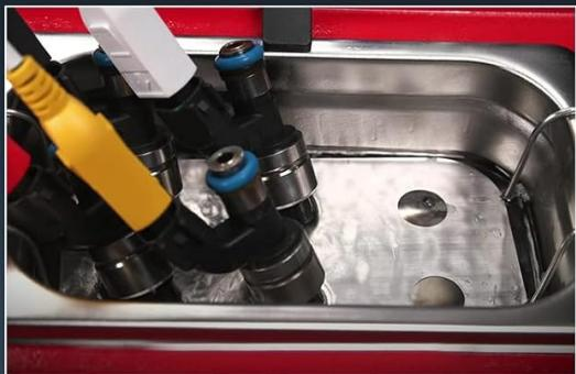
**1** Pour in the detergent and place the fuel injector in the ultrasonic cleaner
