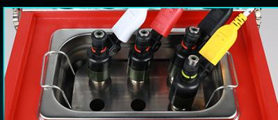
Supports Cleaning of Diesel Injectors
