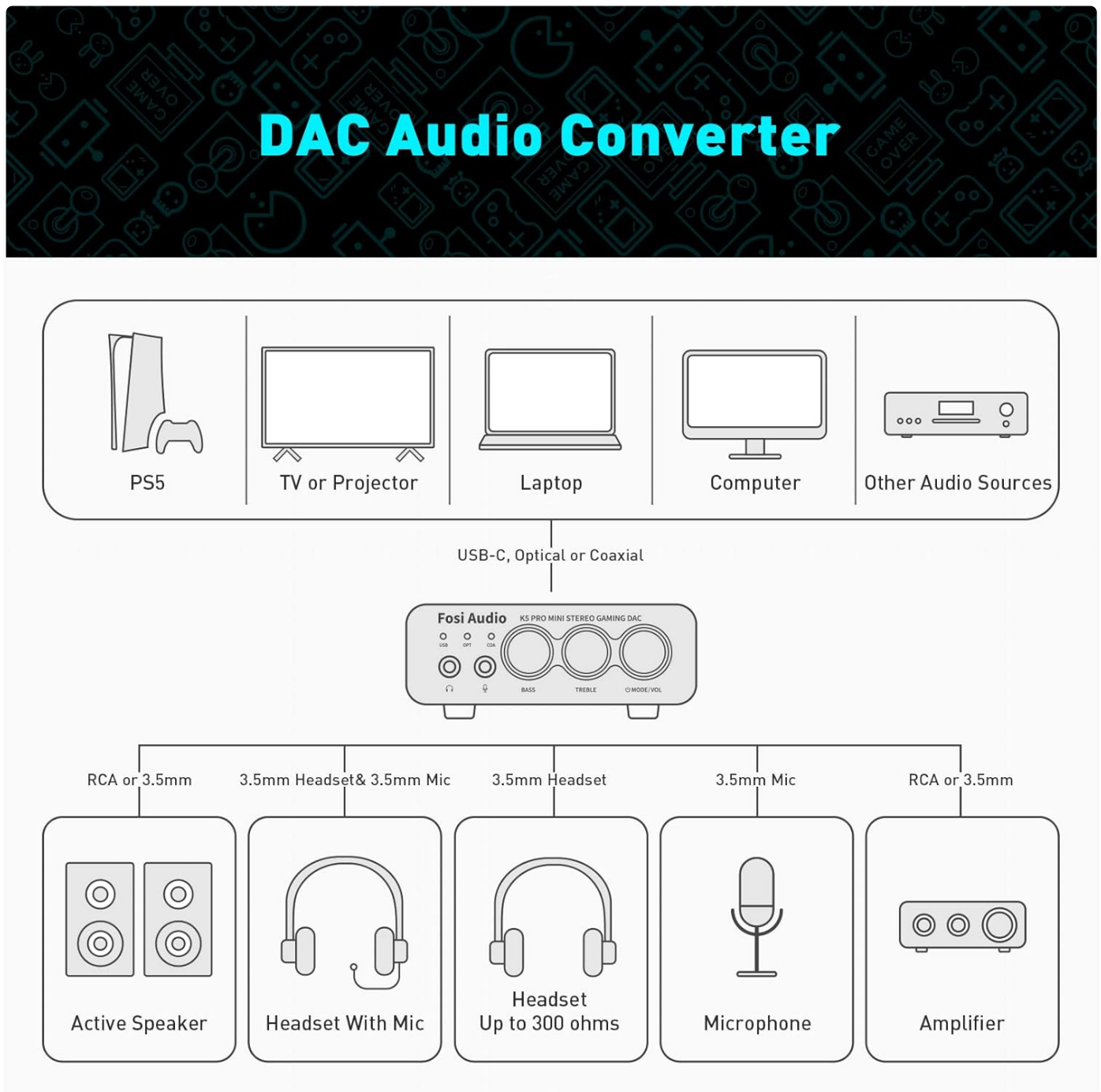
Image 4: A comprehensive diagram illustrating how to connect different audio sources and output devices to the Fosi Audio K5 Pro.
