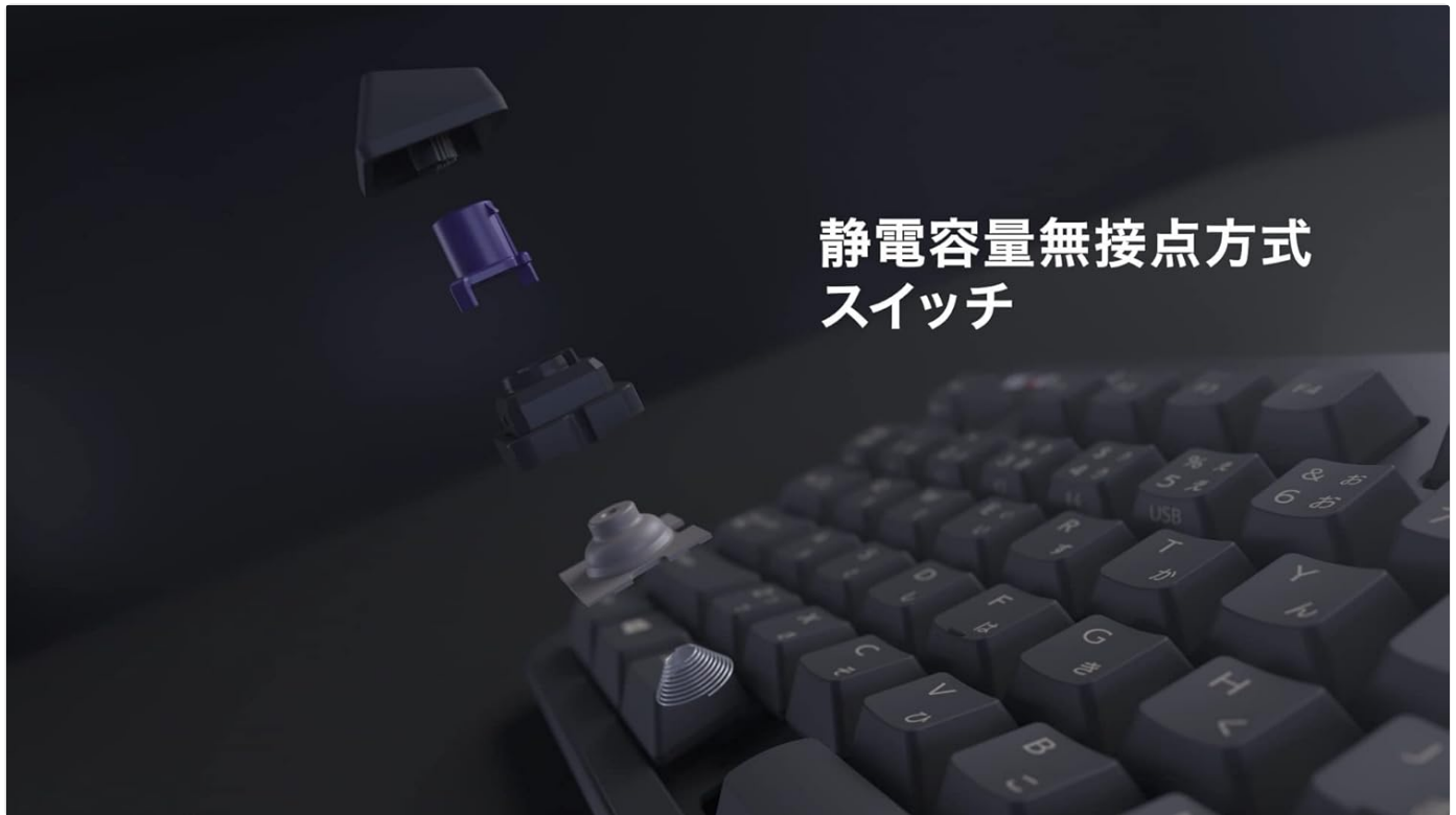
Image: Exploded view of a Tpre switch, illustrating its internal components.
