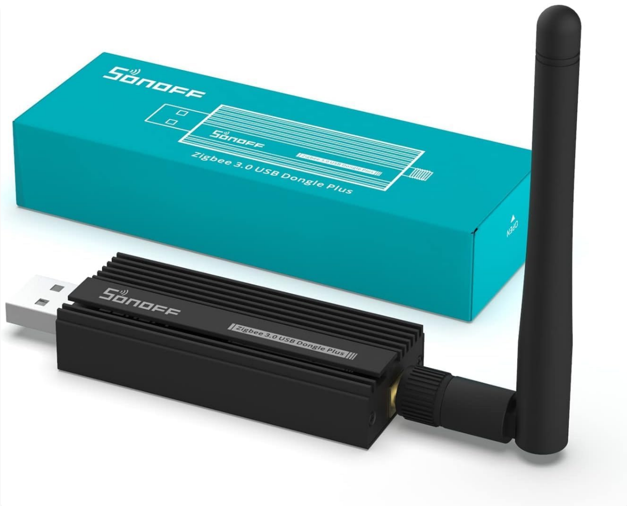
Image 1.1: The SONOFF Zigbee 3.0 USB Dongle Plus, its detachable antenna, and product packaging.
