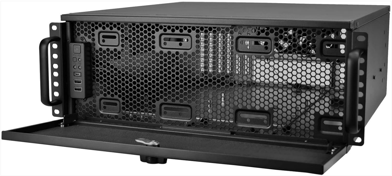
Figure 3.6: The front panel door opened, revealing the power button, reset button, and front I/O ports.
