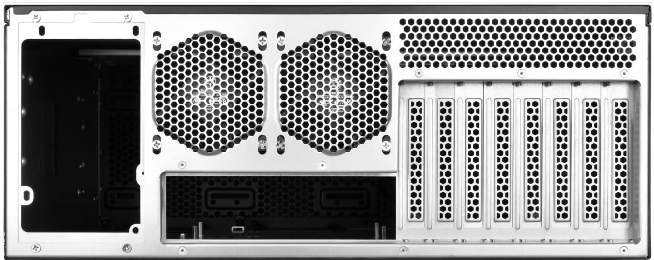
Figure 3.2: Rear view of the RM44 chassis, showing the power supply cutout, fan mounts, and PCIe expansion slots.
