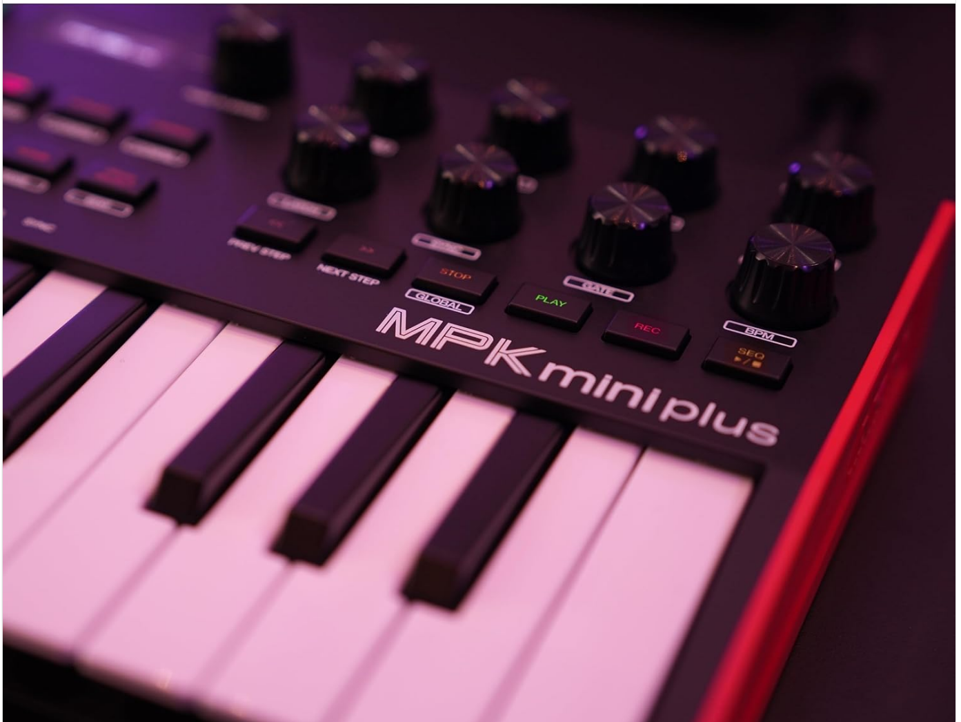
Image: A close-up view of the transport control section on the MPK Mini Plus, highlighting the dedicated buttons for DAW integration.
