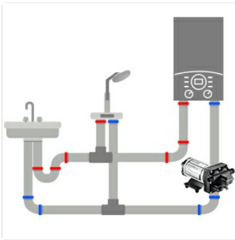
Figure 4.3: Example plumbing diagram illustrating the pump's integration into a typical water system.
