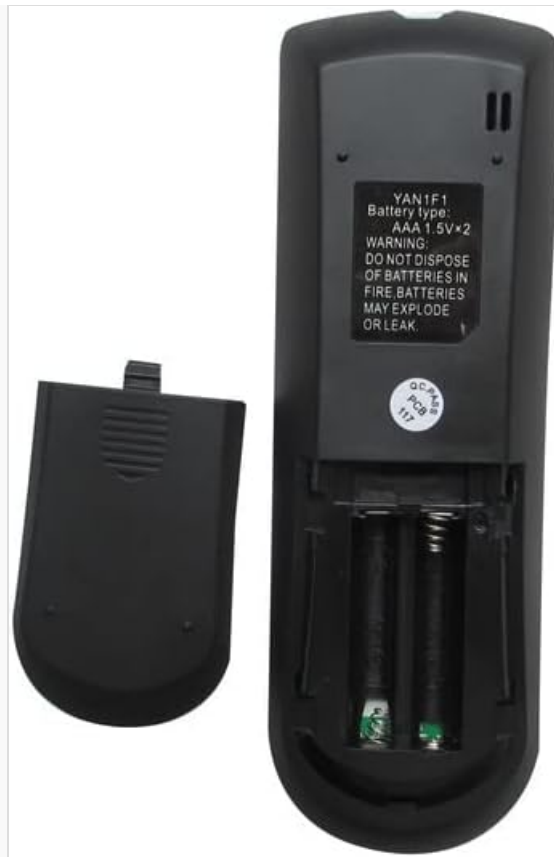
Image: Rear view of the remote control with the battery cover removed, revealing the two AAA battery slots. This illustrates where to insert the batteries.
