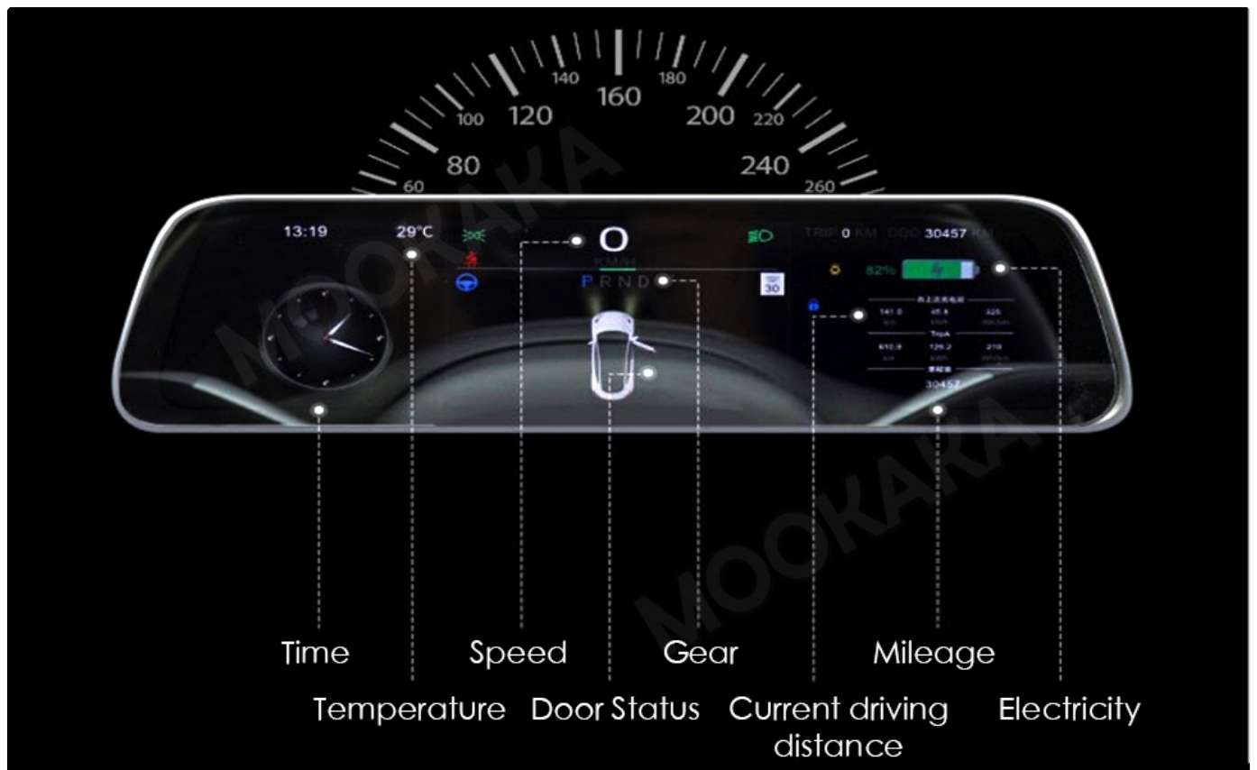
Image 5.2: A detailed diagram highlighting the specific data points presented on the MOOKAKA display for comprehensive driver information.
