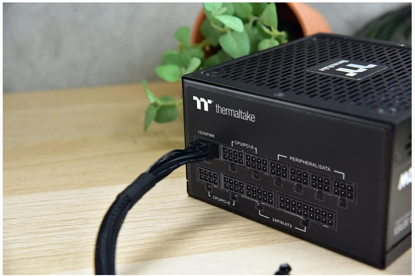
Figure 4: Detailed view of the fully modular cable connection ports on the power supply, including the 12VHPWR connector.
