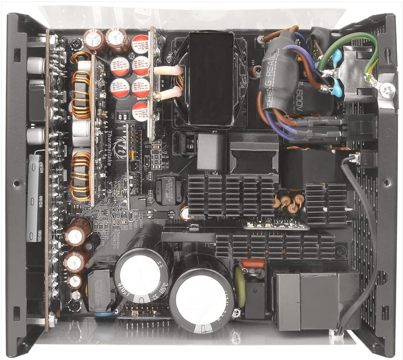
Figure 9: Internal view of the power supply, showcasing the high-quality Japanese capacitors and other premium components.
