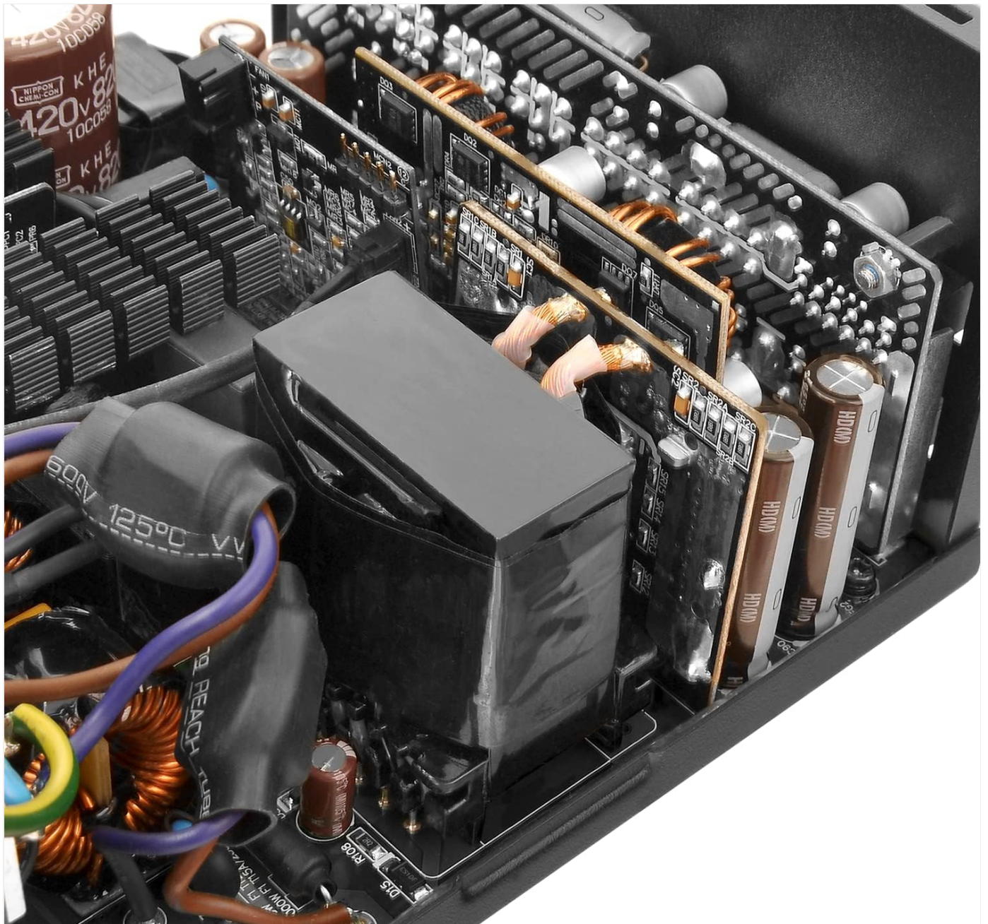
Figure 8.2: Internal view of the power supply's main PCB and components.
