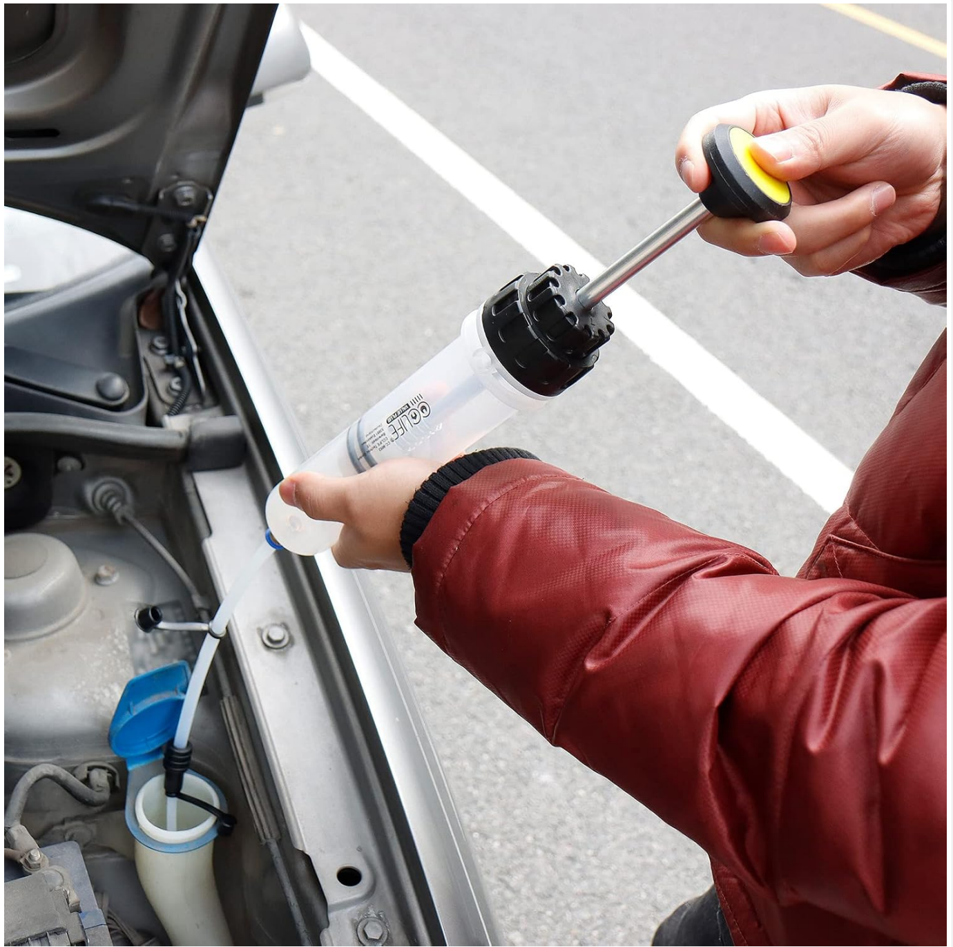
Figure 6.2: Example of using the CCLIFE fluid extractor to add new windshield washer fluid to a vehicle's reservoir.
