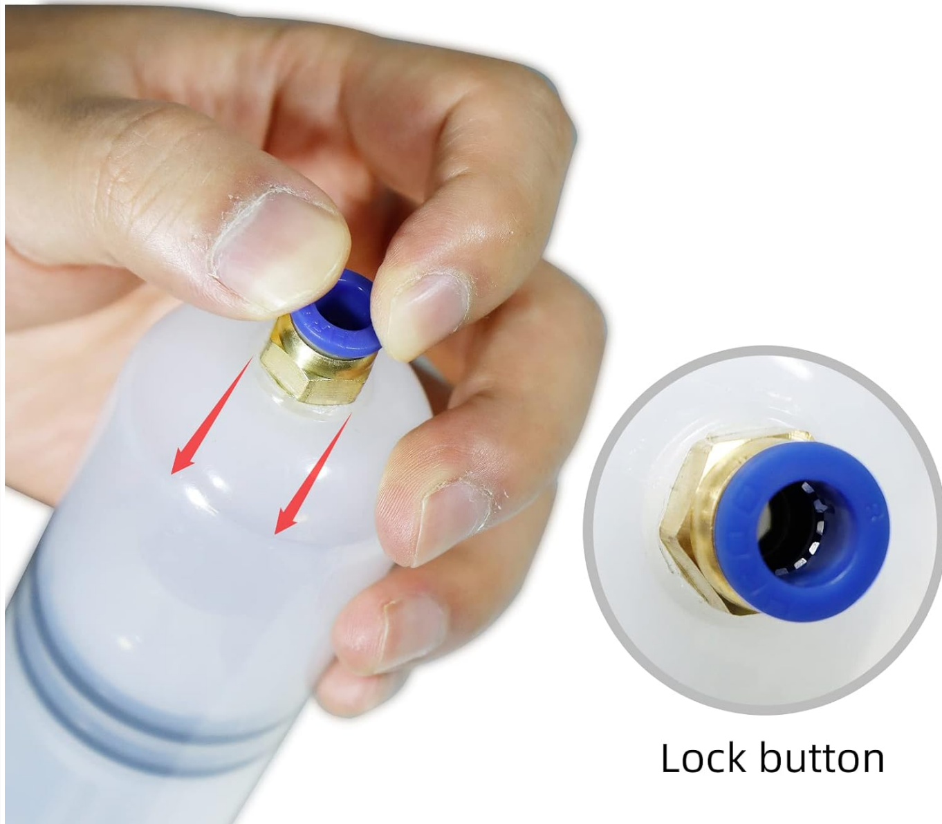
Figure 5.1: Illustration demonstrating how to connect or disconnect the hose by pressing the blue lock button on the pump's connector.
