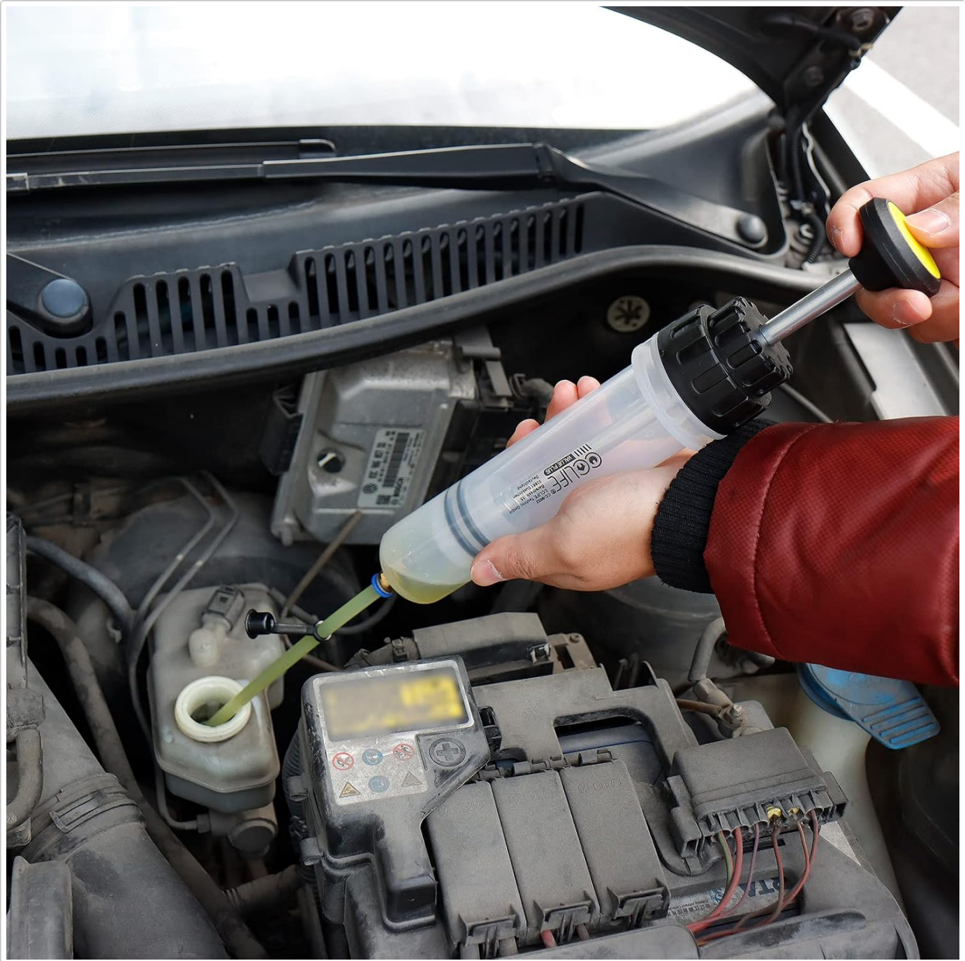
Figure 6.1: Example of using the CCLIFE fluid extractor to remove old brake fluid from a vehicle's master cylinder reservoir.
