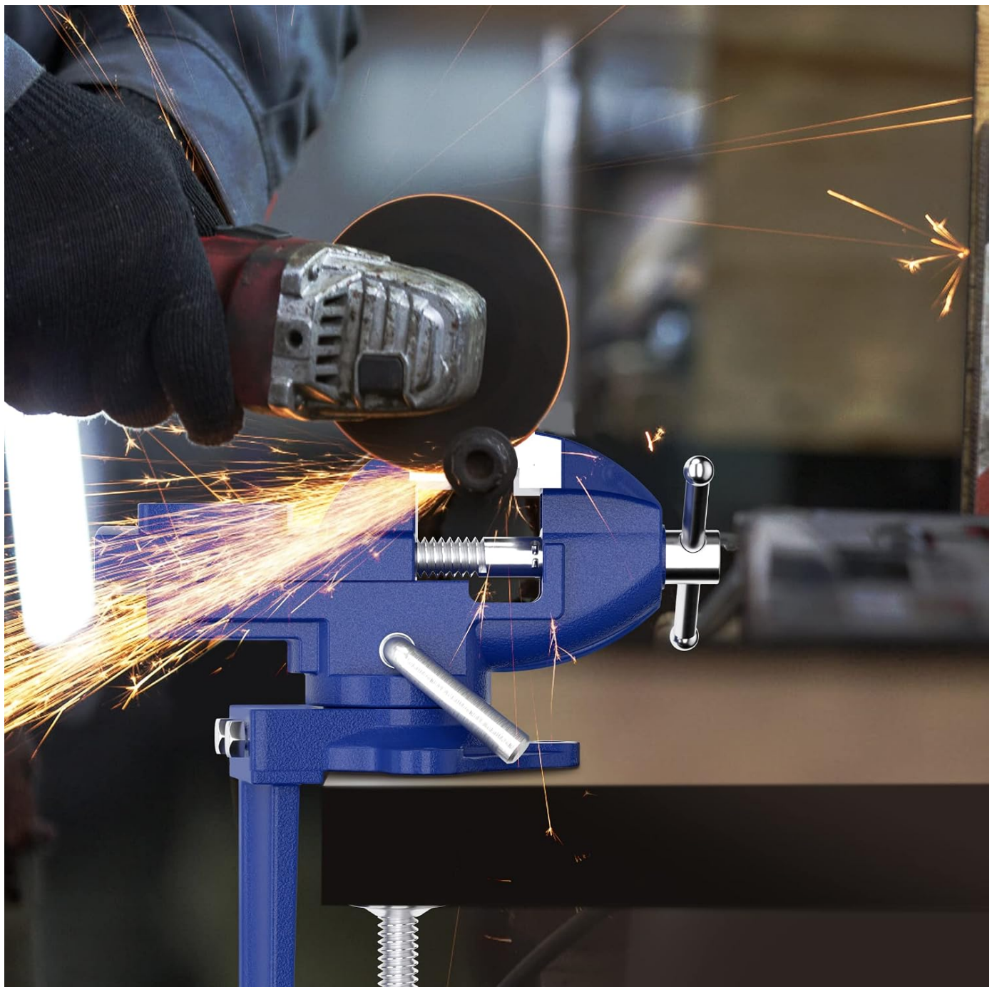
Figure 4.1: The vise securely holds a workpiece during metalworking tasks.
