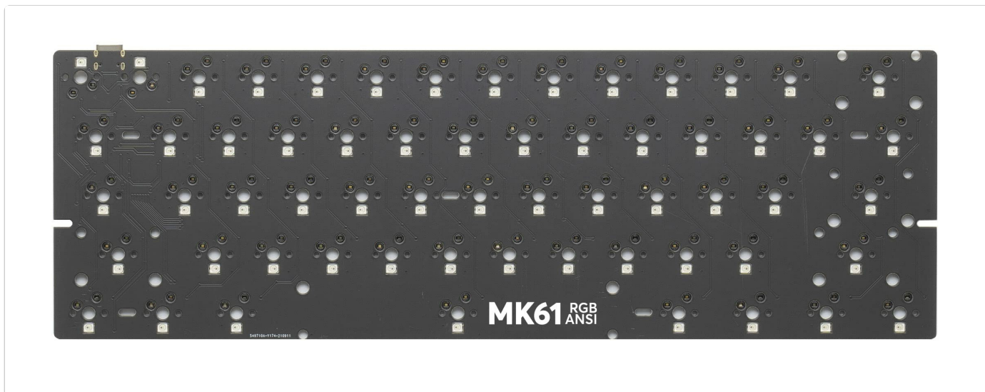
Image: The MK MK61 Hotswap PCB, featuring Kailh hotswap sockets for easy switch installation and individual SMD LEDs for per-key RGB backlighting. The USB-C port is visible on the top right edge.
