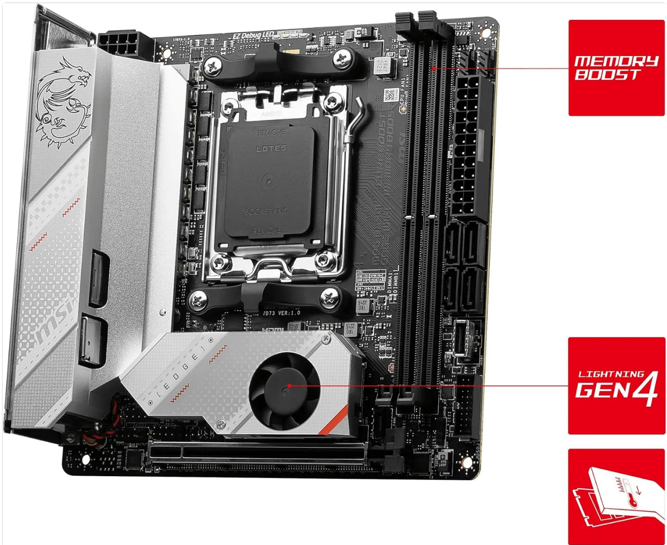
Figure 3: An angled view of the motherboard, highlighting the two DDR5 memory slots and the M.2 cooling fan.
