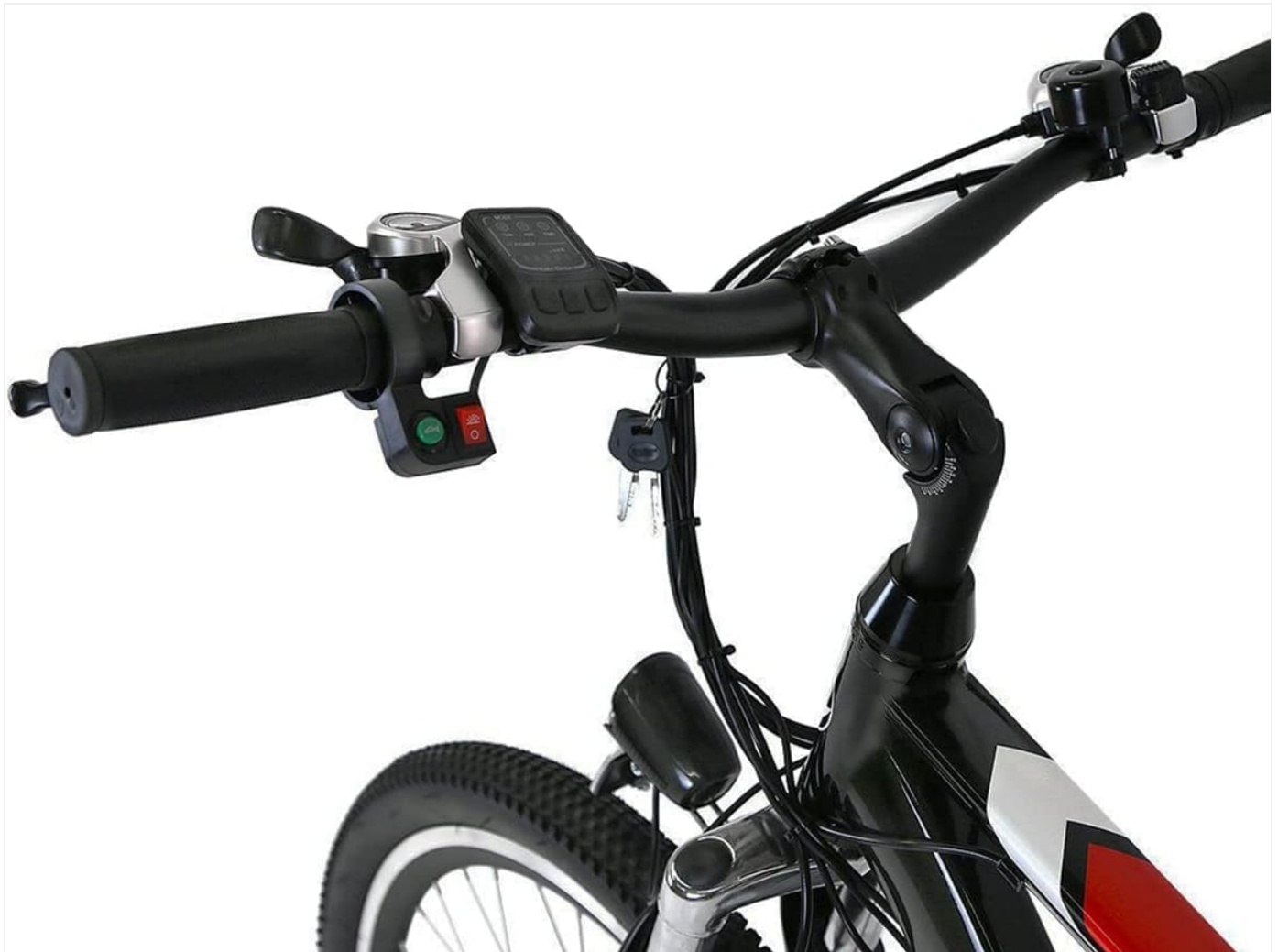
Figure 4.1: Close-up view of the handlebar controls. This image displays the grip, brake levers, gear shifter, and the control panel for the electric assist system.
