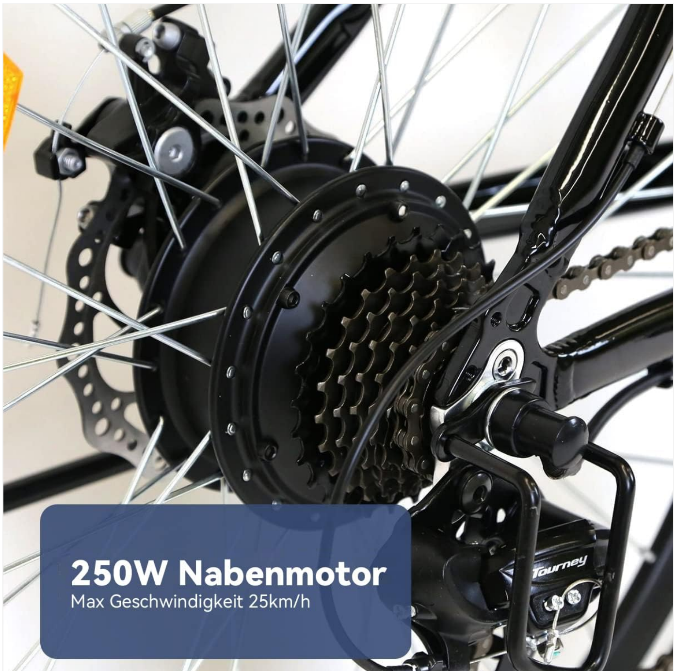
Figure 4.2: Detail of the rear wheel, showing the 250W hub motor and the Shimano 7-speed drivetrain. The disc brake rotor is also visible.
