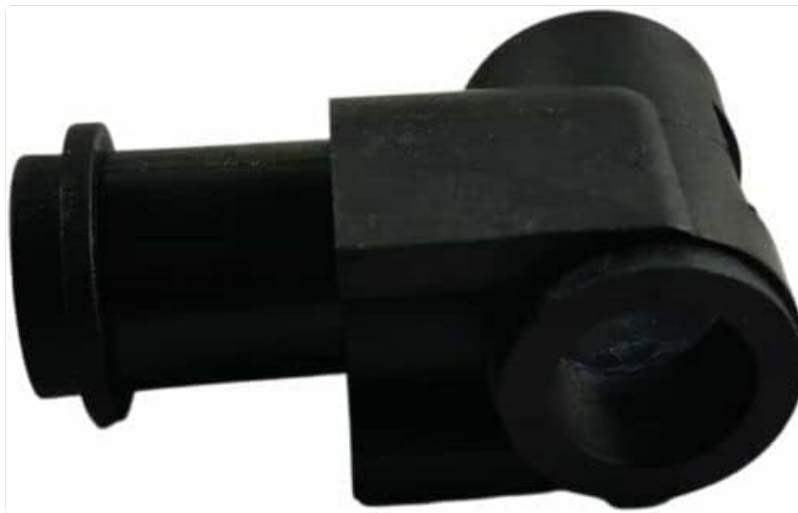
Figure 2: EFP Steering Shaft Support from a side perspective, illustrating the shaft opening and overall dimensions.
