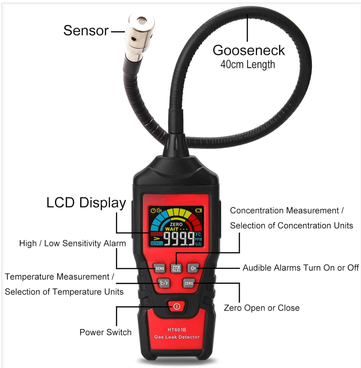
Figure 3.1: HT601B Gas Leak Detector with labeled parts. Key components include the sensor at the tip of the 40cm gooseneck, the LCD display, and buttons for sensitivity adjustment, unit selection (PPM/LEL), audible alarm control, zeroing, and power.
