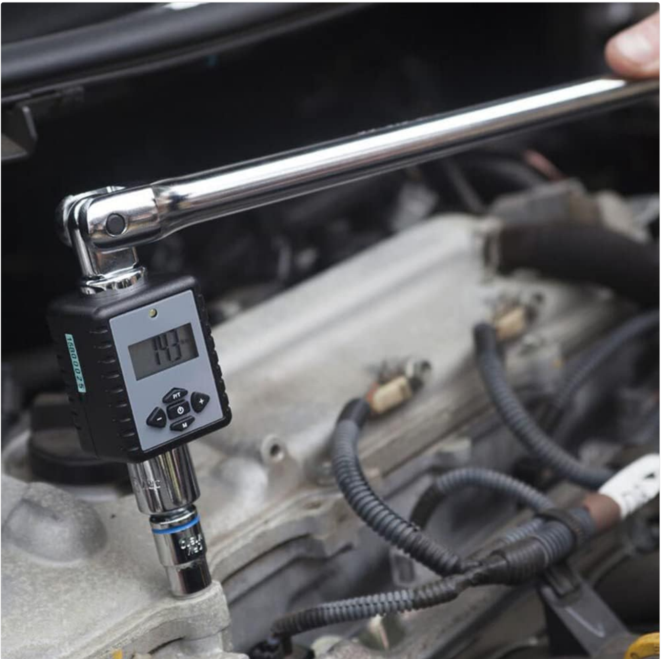
Figure 5.1: Adapter in Use. The image shows the digital torque adapter connected to a ratchet wrench, being used to tighten a fastener on an engine.
