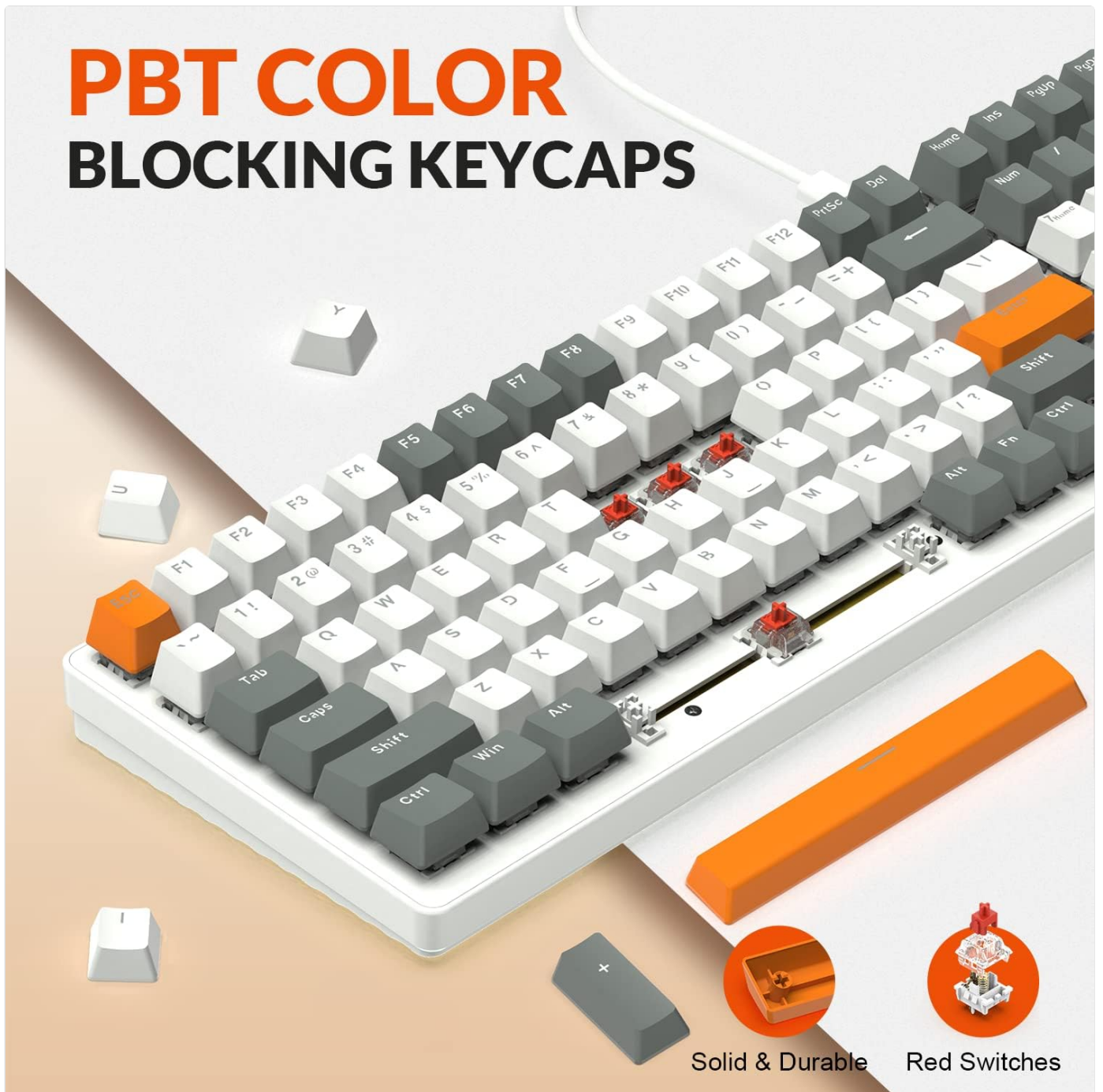
Image: A detailed view of the K3 keyboard's PBT color-blocking keycaps and the underlying red switches, illustrating the hot-swappable design and durable keycap material.
