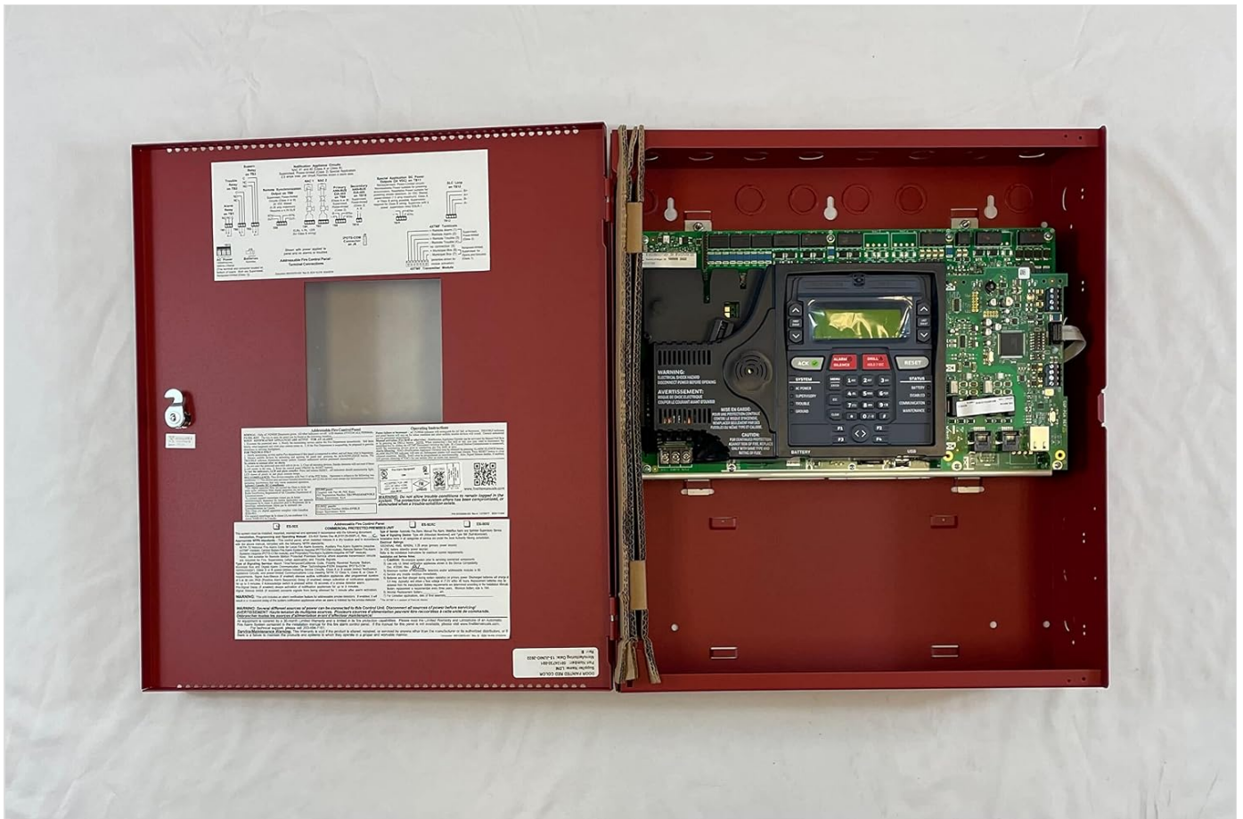
Image: The ES-50X FACP with its enclosure open, showing the internal components, main circuit board, and the user interface panel.
