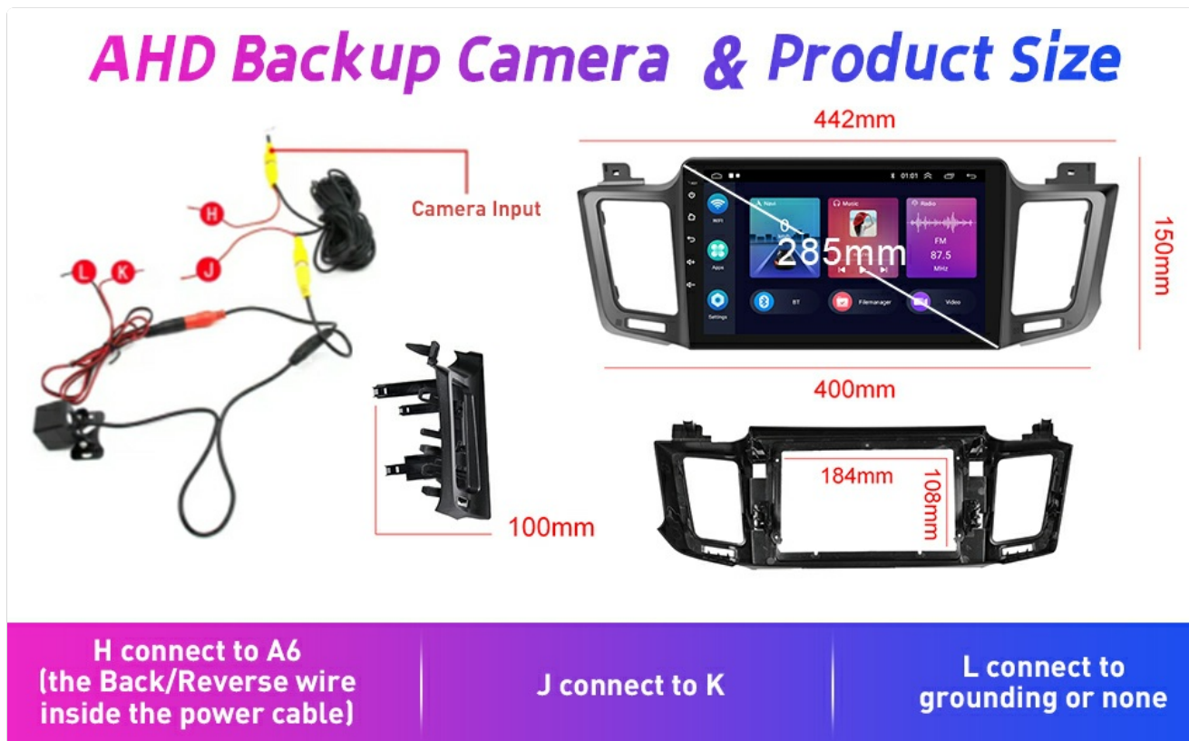
Figure 5.2: This image displays the wiring for the AHD backup camera, indicating connections for the reverse wire (A6), power (K), and ground (L). It also shows the dimensions of the Roinvou car stereo unit.
