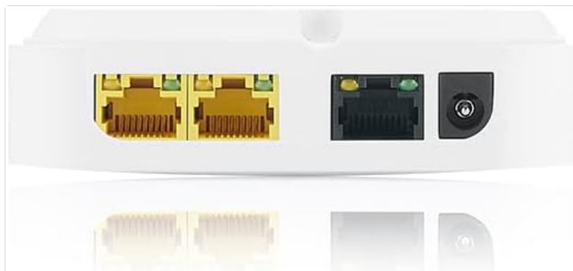
Figure 2: Rear view of the Zyxel WAC500H Access Point, highlighting the two Gigabit Ethernet ports (one with PoE) and the power input.
