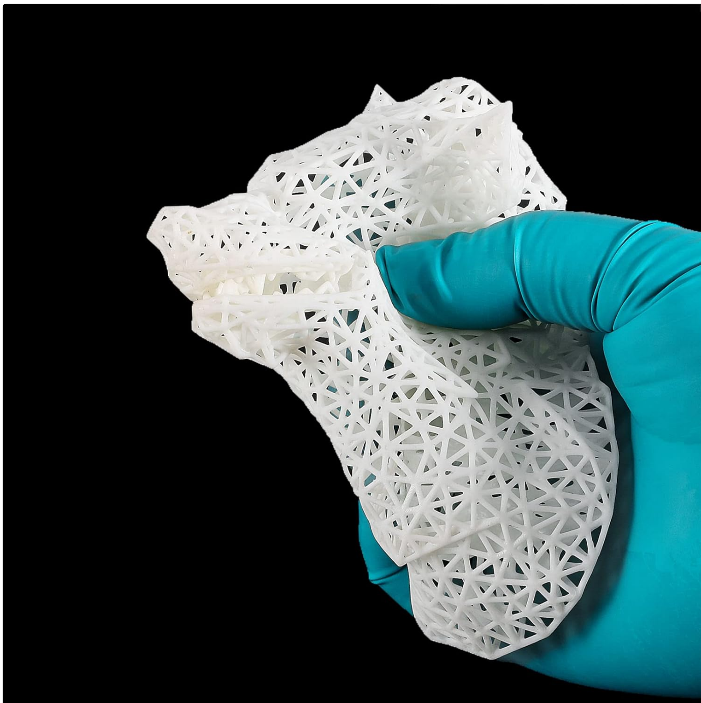
Image: A flexible lattice structure printed with F39 resin, demonstrating its soft and pliable nature.
