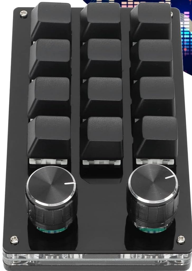
Image 5.1: The macro pad knobs can be programmed for media and navigation controls.
