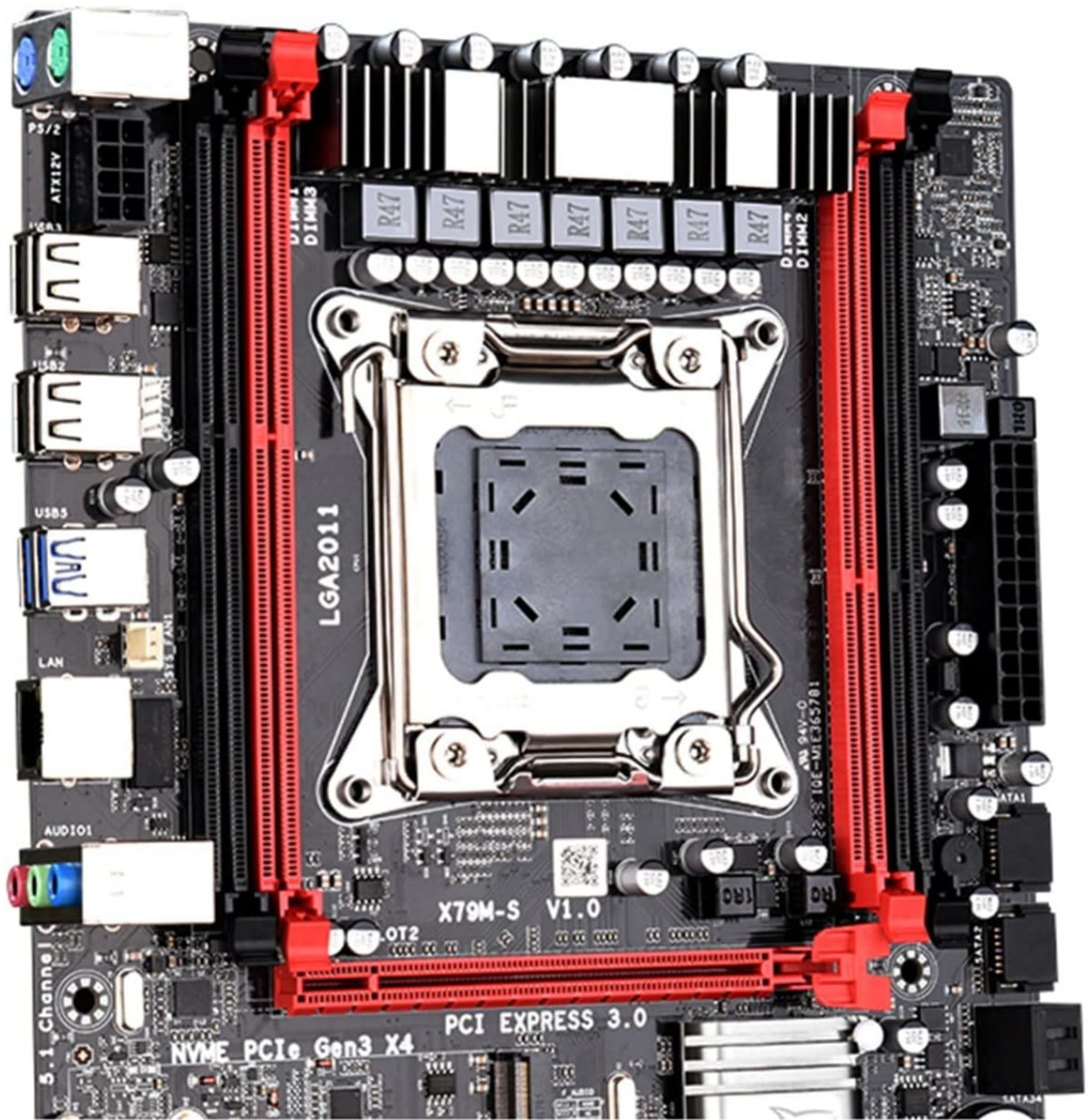
Figure 1.1: Front view of the JINGSHA X79M-S 3.0 ATX Motherboard, showcasing the LGA2011 CPU socket, DDR3 memory slots, and PCI Express slots.
