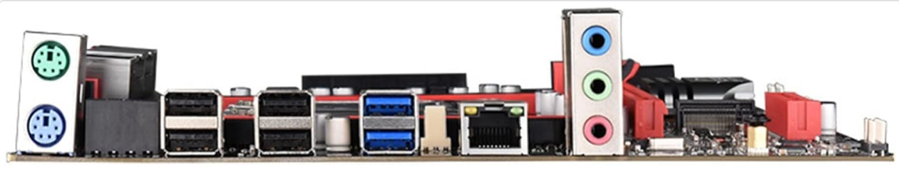
Figure 2.2: Rear I/O panel of the motherboard, showing PS/2 ports for mouse and keyboard, USB 2.0 and USB 3.0 ports, Gigabit Ethernet port, and audio jacks.
