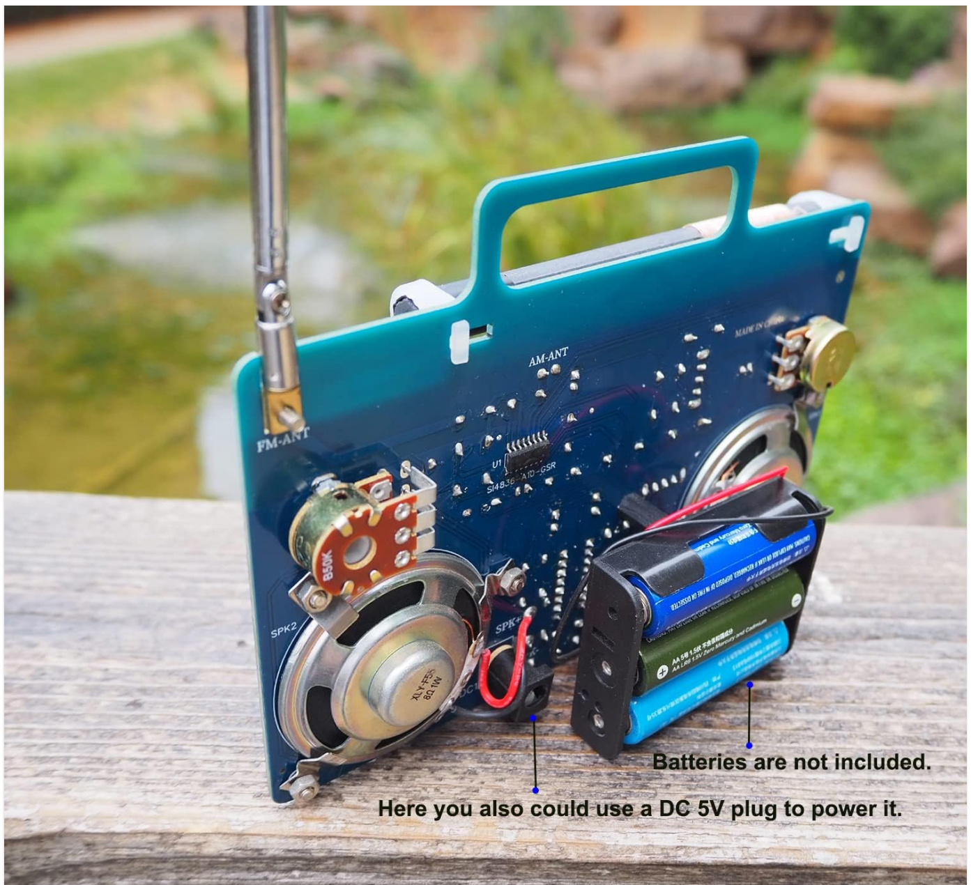
Image: Rear view of the assembled radio, highlighting the battery compartment for 3 AA batteries and the DC 5V plug input for alternative power.
