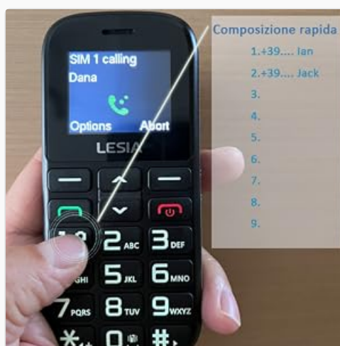
Image 4.2: Demonstrating the use of speed dial for quick access to contacts.
