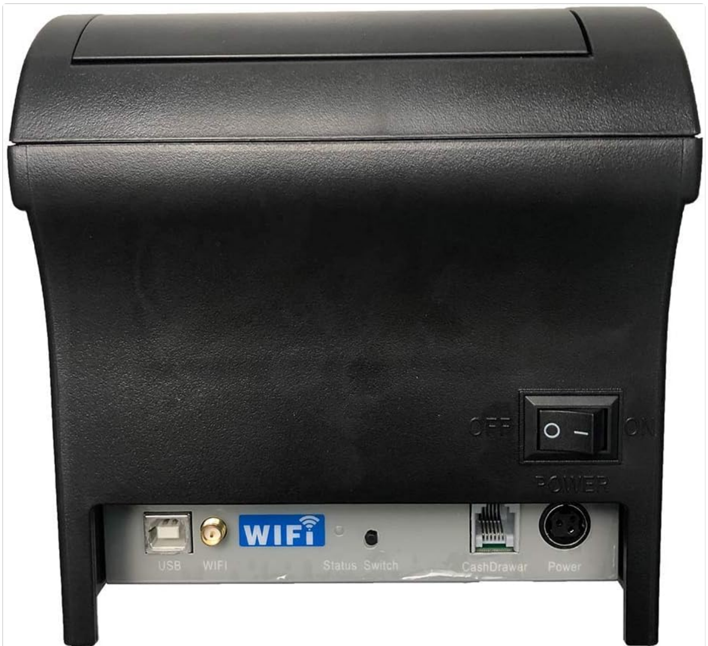
Image: Rear view of the NETUM thermal printer, highlighting the various connectivity ports including USB, WiFi antenna port, Status
