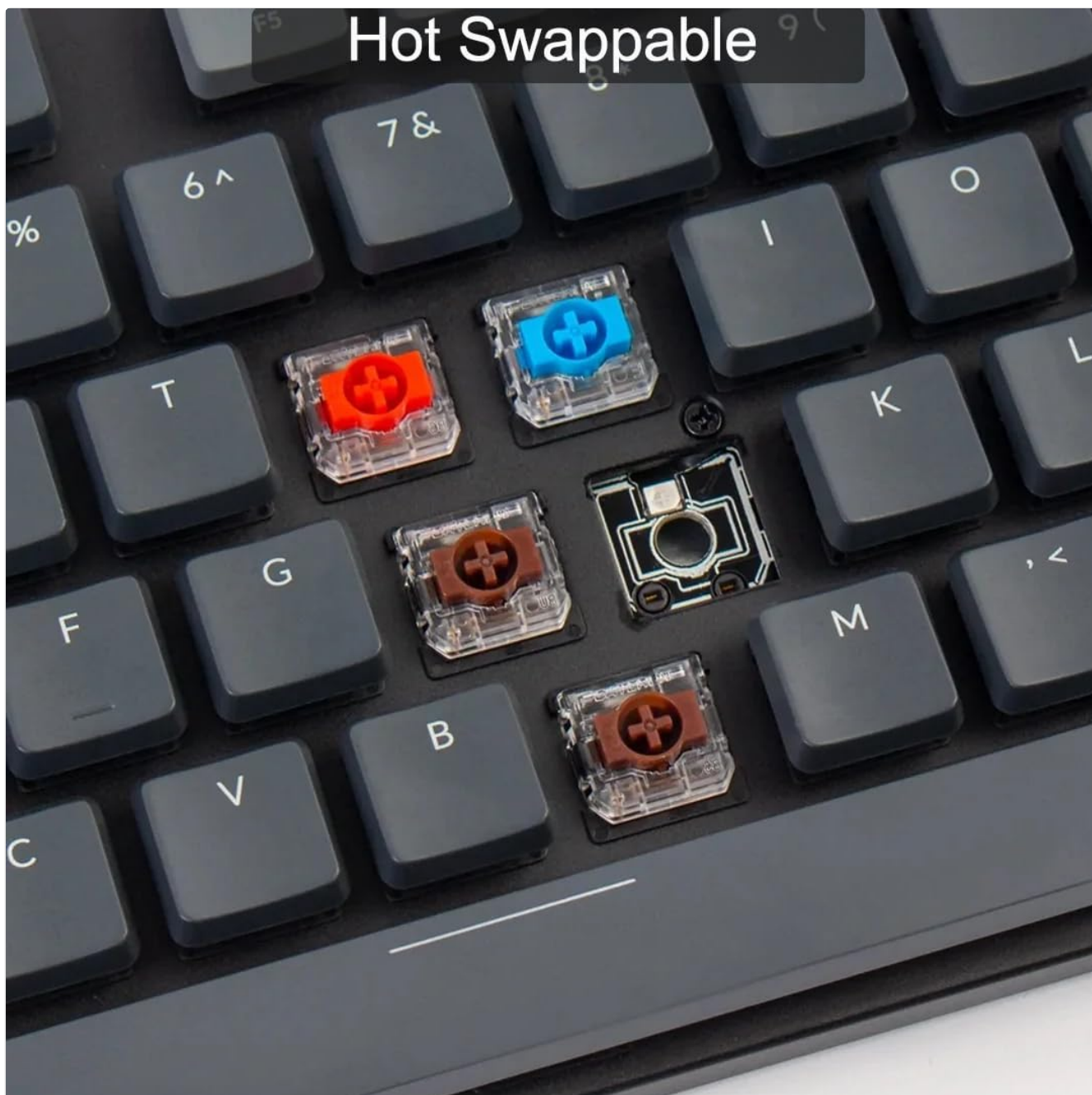
Image: A close-up view of the Keychron K5 SE keyboard with some keycaps removed, revealing the hot-swappable Gateron mechanical switches in various colors (red, blue, brown). This demonstrates the ease of customizing the typing experience.
