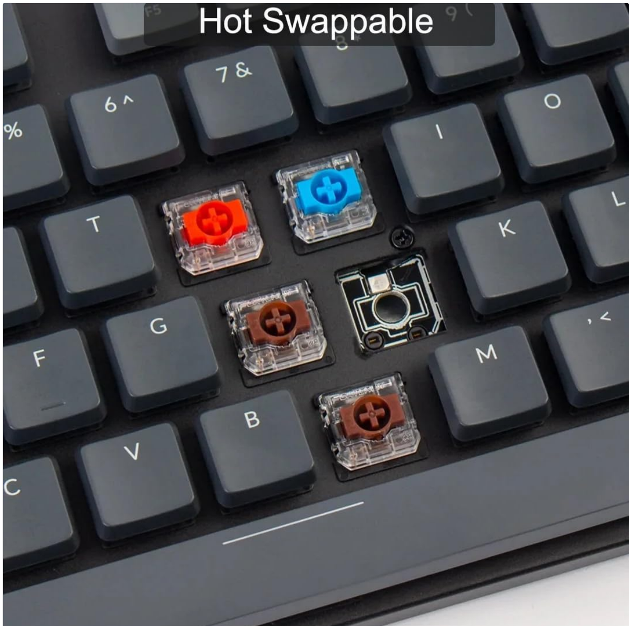
Image: A detailed view of the Keychron K5 SE keyboard's hot-swappable switch sockets, with several keycaps and switches removed to illustrate the ease of customization.
