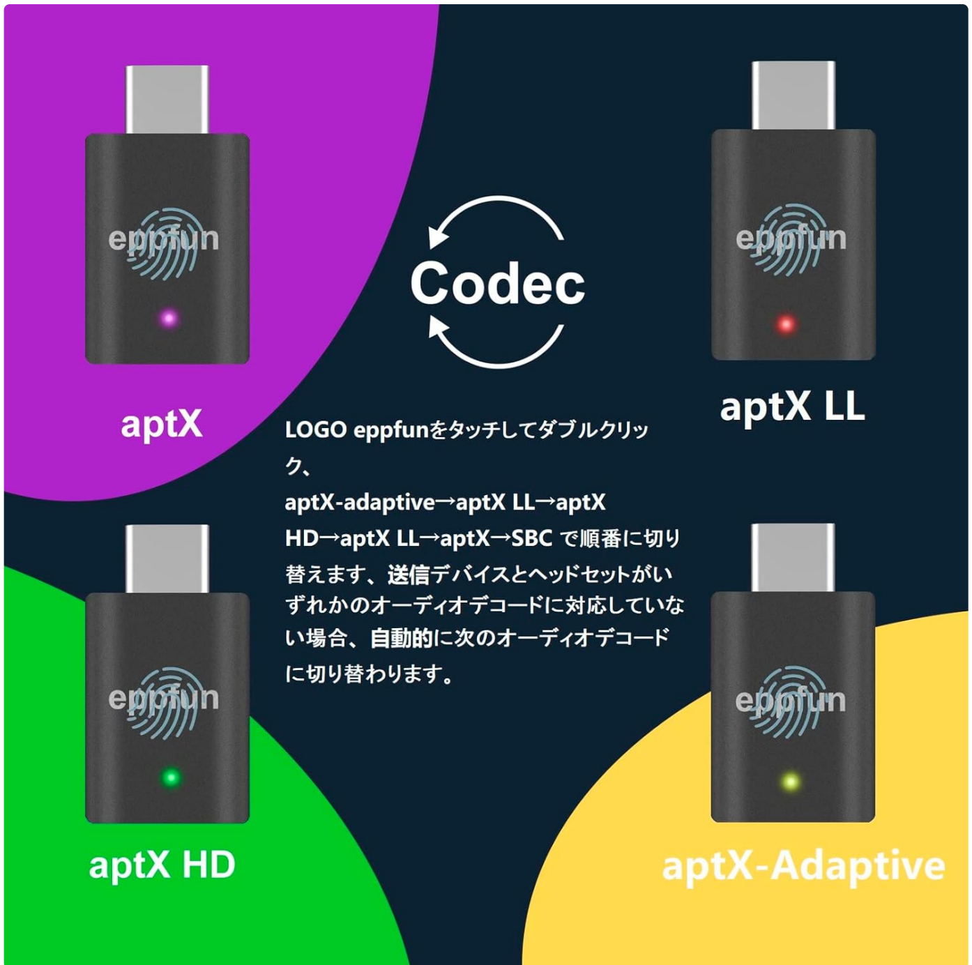
Image: A visual representation of the codec switching process and the corresponding LED colors for each audio mode.
