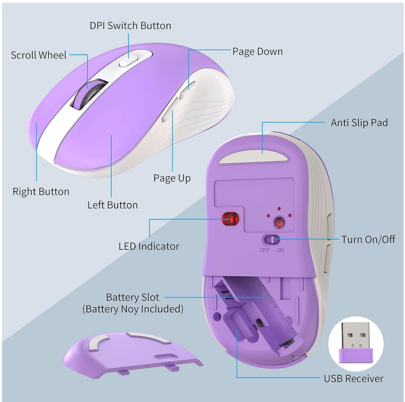
Image 2.3: A detailed diagram of the mouse, indicating the scroll wheel, buttons, LED indicator, battery slot, and USB receiver storage.
