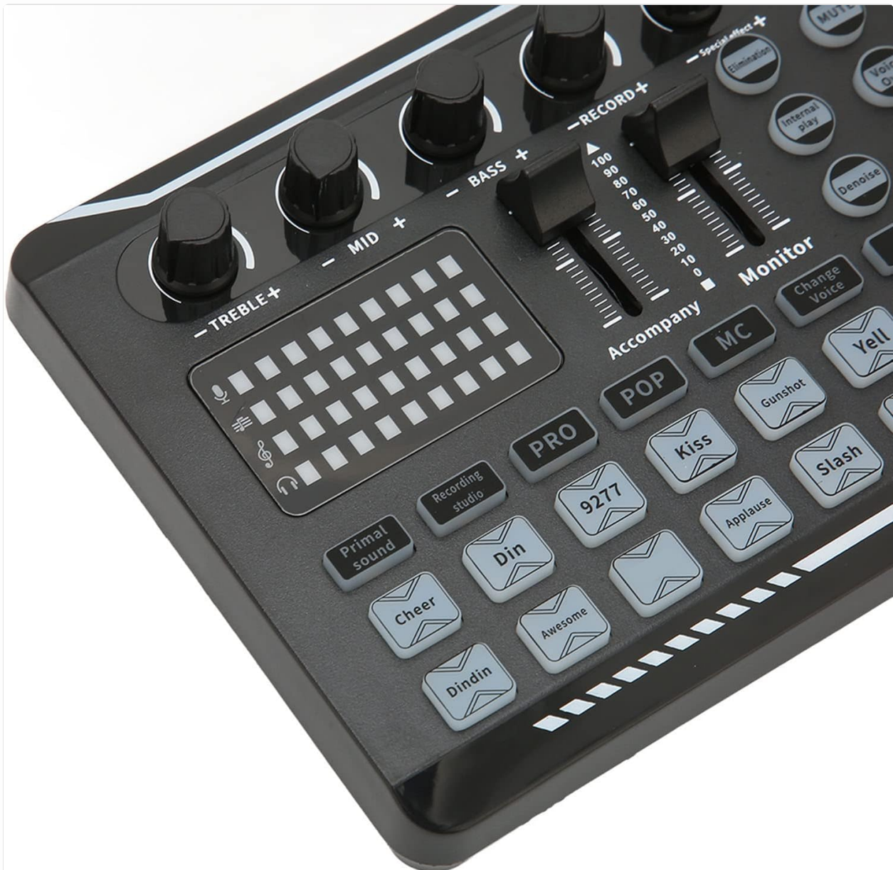
Image: A detailed view of the left side of the sound card, showing the Treble, Mid, and Bass adjustment knobs, the Accompany and Monitor faders, and a grid of special effect buttons.
