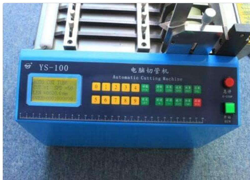
Figure 3.2: Close-up of the YS-100 control panel. The panel features an LCD display, numerical keypad, function buttons (green and red), and emergency stop button (red circular button).
