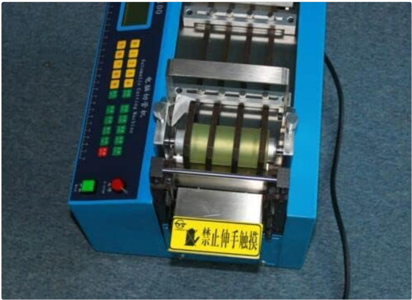
Figure 3.3: View of the material feed and cutting mechanism. This area includes rollers for material advancement and the cold cutting blade. A yellow warning label is visible, indicating to keep hands clear.
