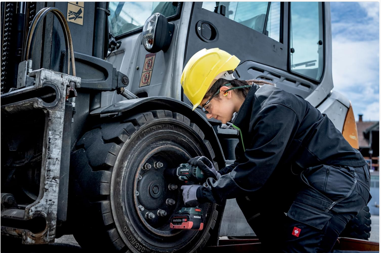
Figure 6: A worker using the Metabo impact wrench to remove lug nuts from a vehicle tire. This showcases the tool's efficiency and power for automotive maintenance tasks.
