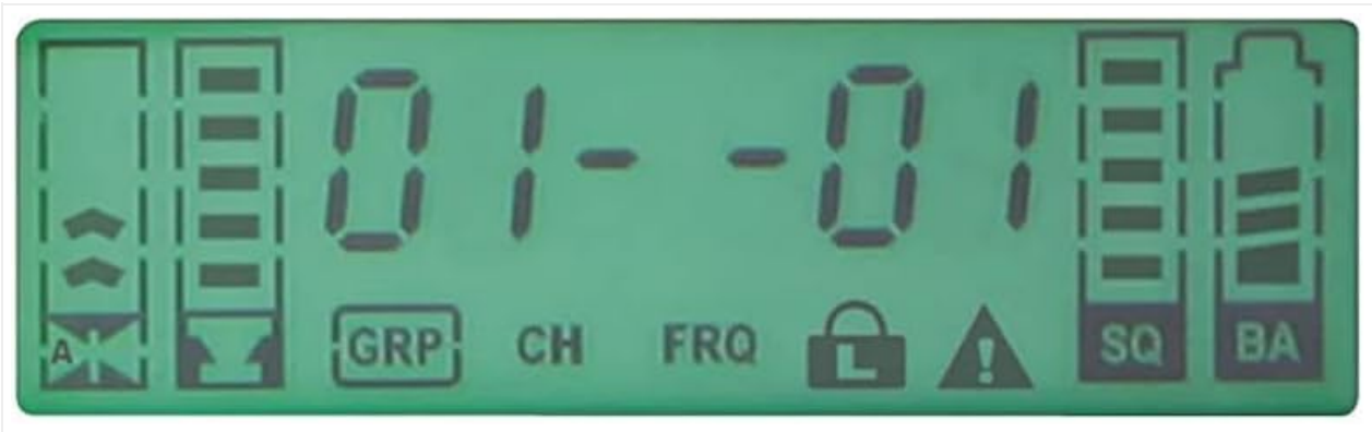
Figure 4: Close-up view of the Mipro ACT-311B Receiver's LCD display, showing channel, group, frequency, and battery indicators.
