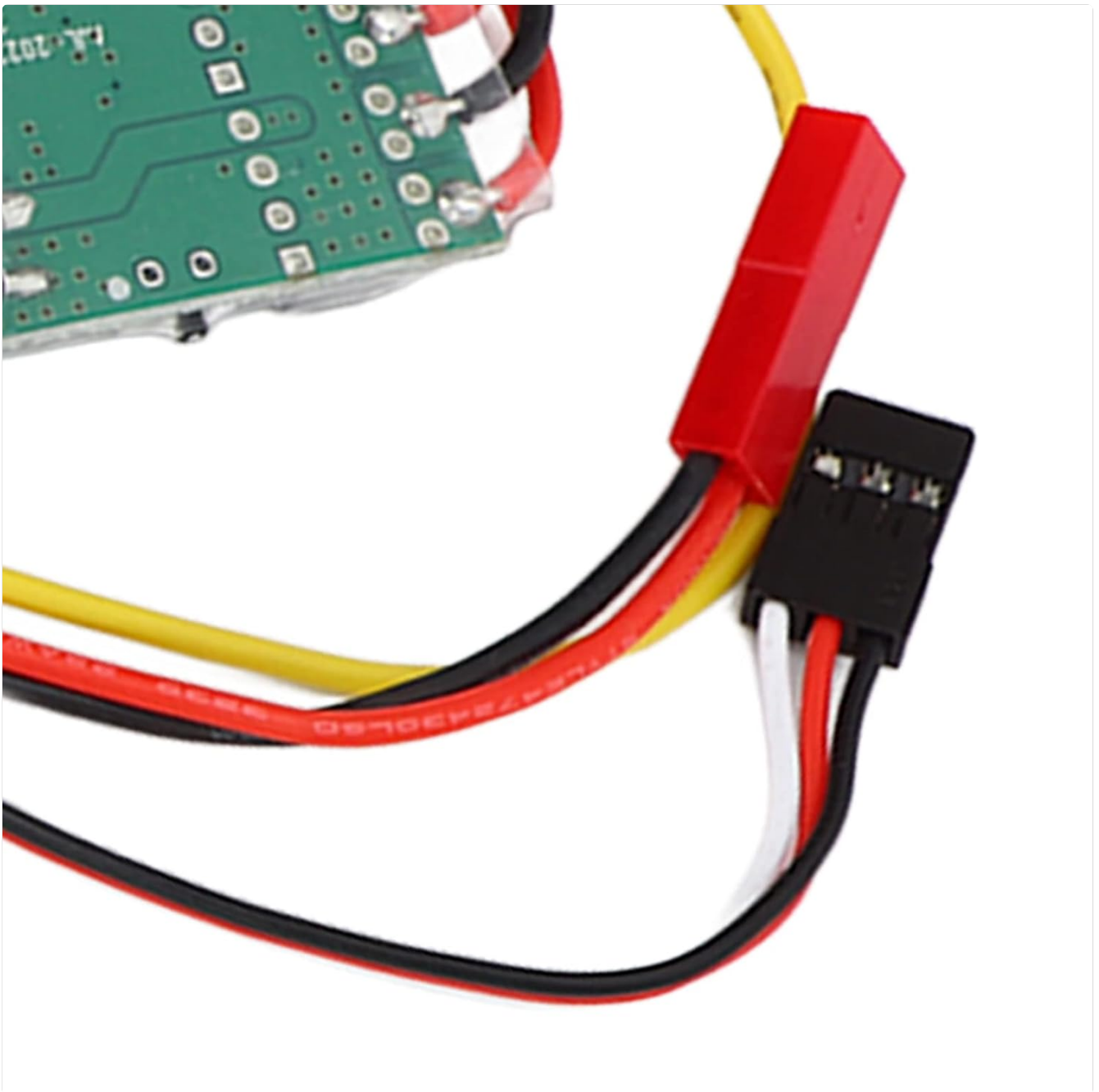
Figure 3: Detailed view of the ESC connectors for receiver and power input.
