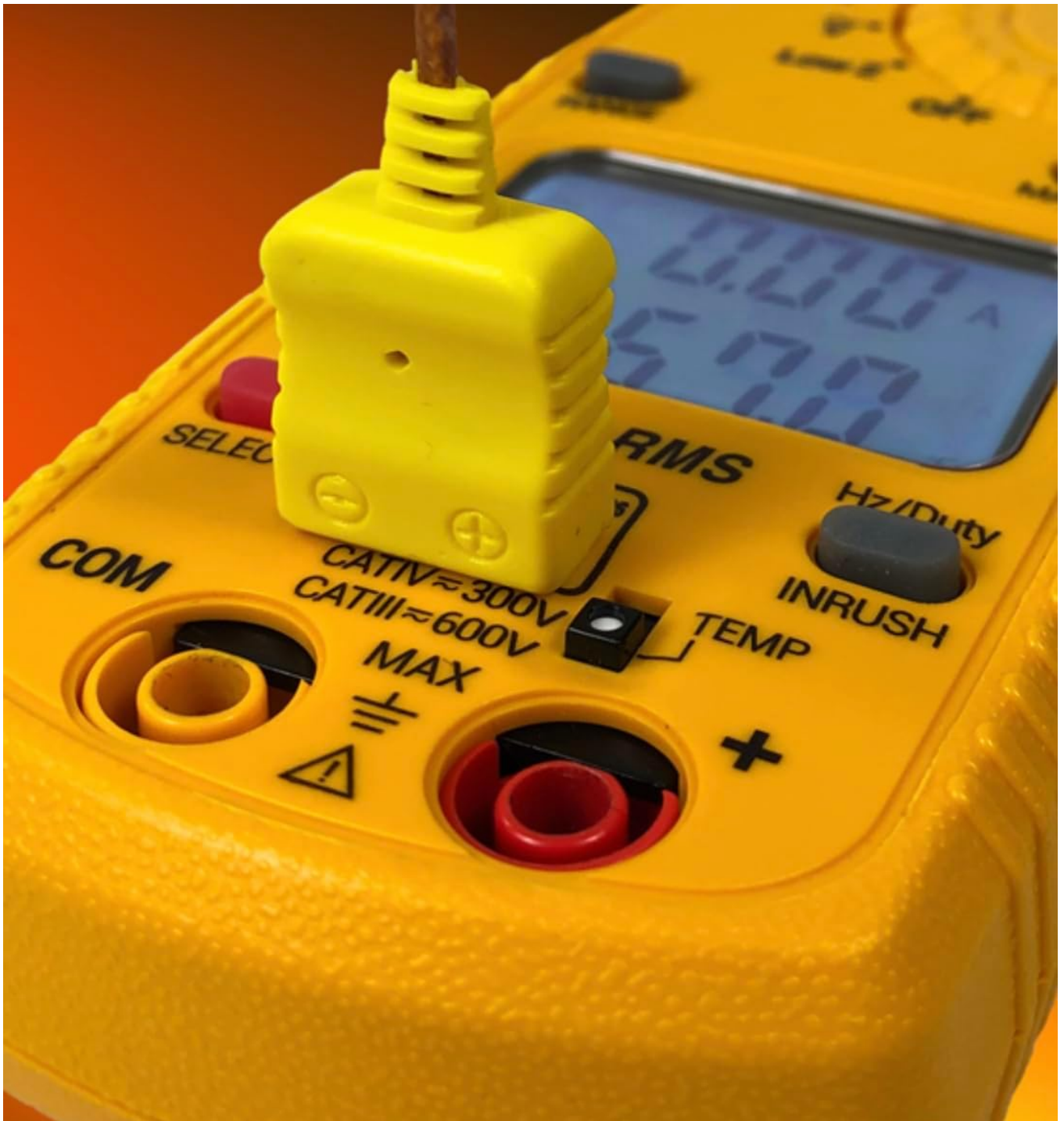
Figure 4: Detail of the test lead input jacks and the K-Type temperature probe input, with a probe connected.
