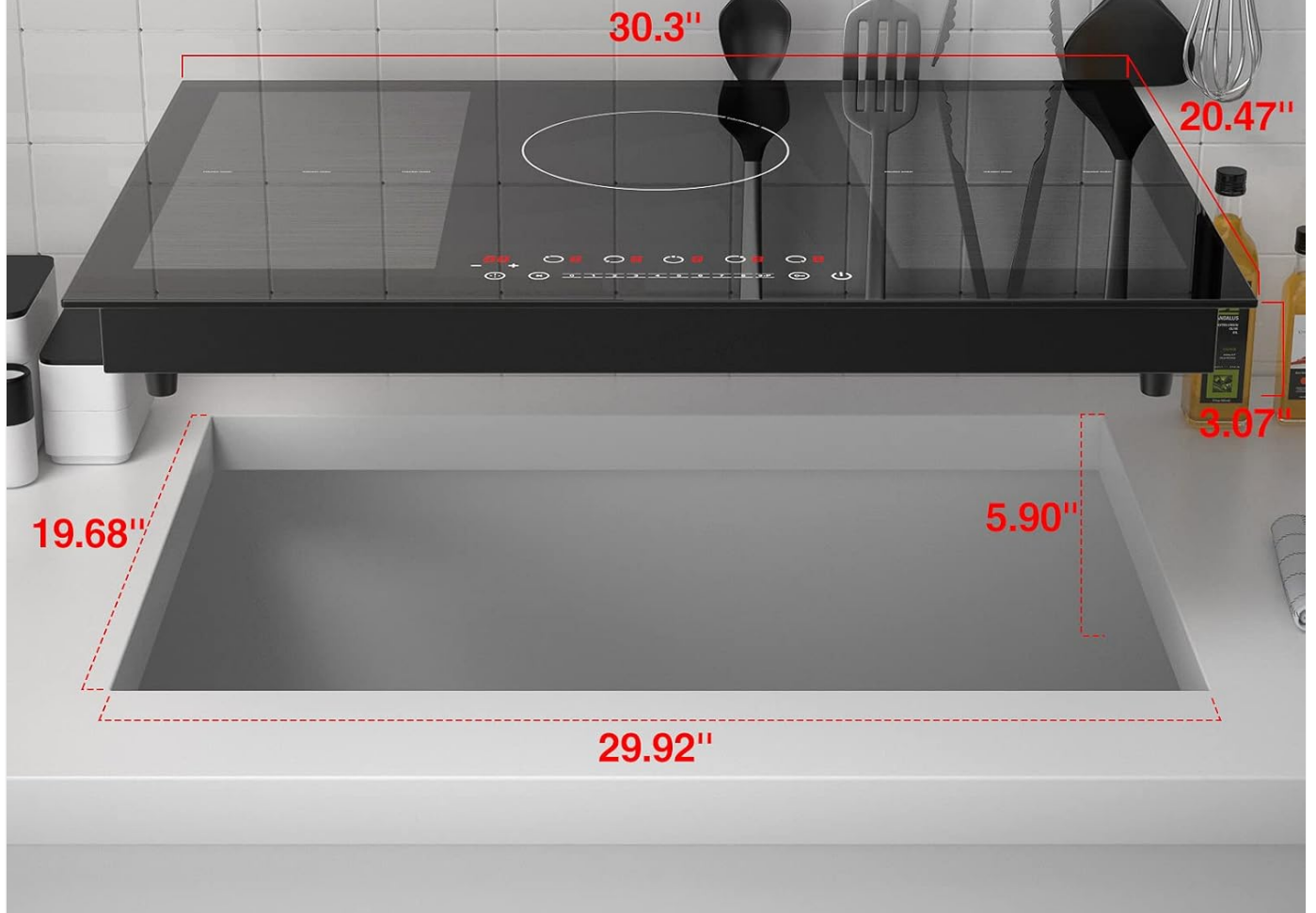
Figure 5: Built-in dimensions and installation guide.
