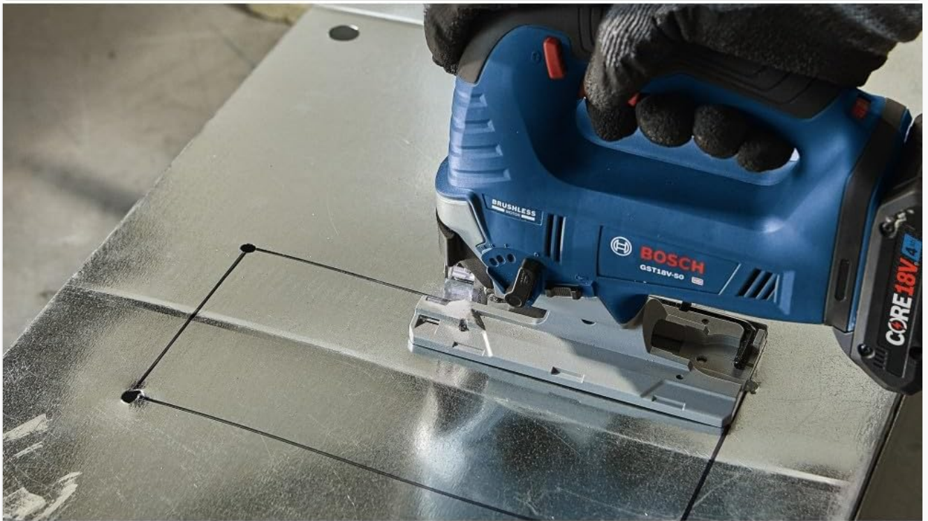
Figure 5: The jig saw is capable of cutting various materials, including metal sheets.
