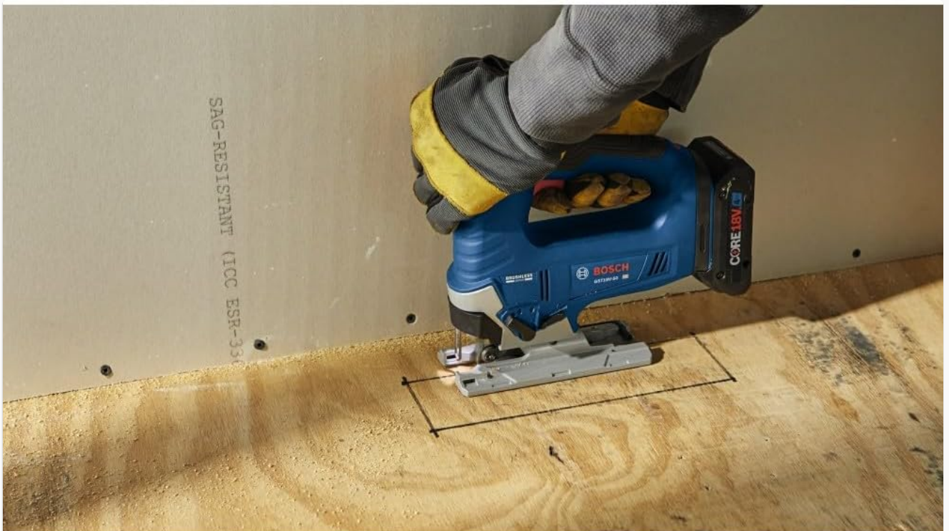
Figure 6: The dust blower mechanism helps keep the cut line clear of sawdust.
