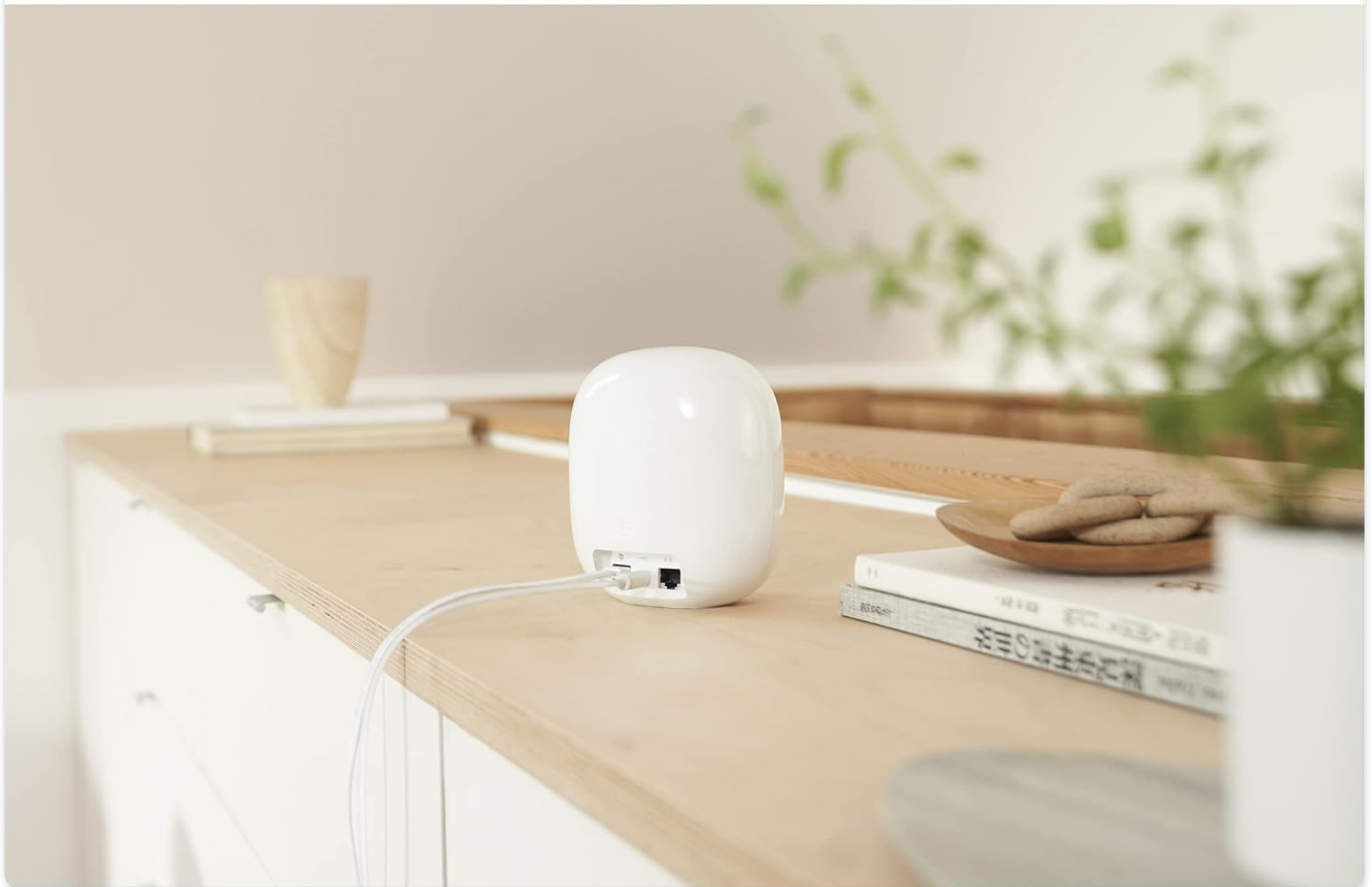
Image: Rear view of a Nest Wifi Pro unit, highlighting its Ethernet ports for input and output, and the power connection.
