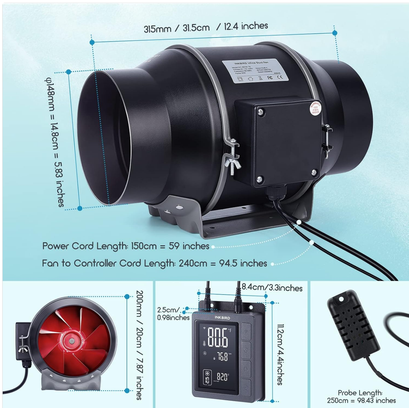
Figure 2.1: Overview of the Inkbird Inline Duct Fan and its components, including dimensions of the fan, controller, and probe.
