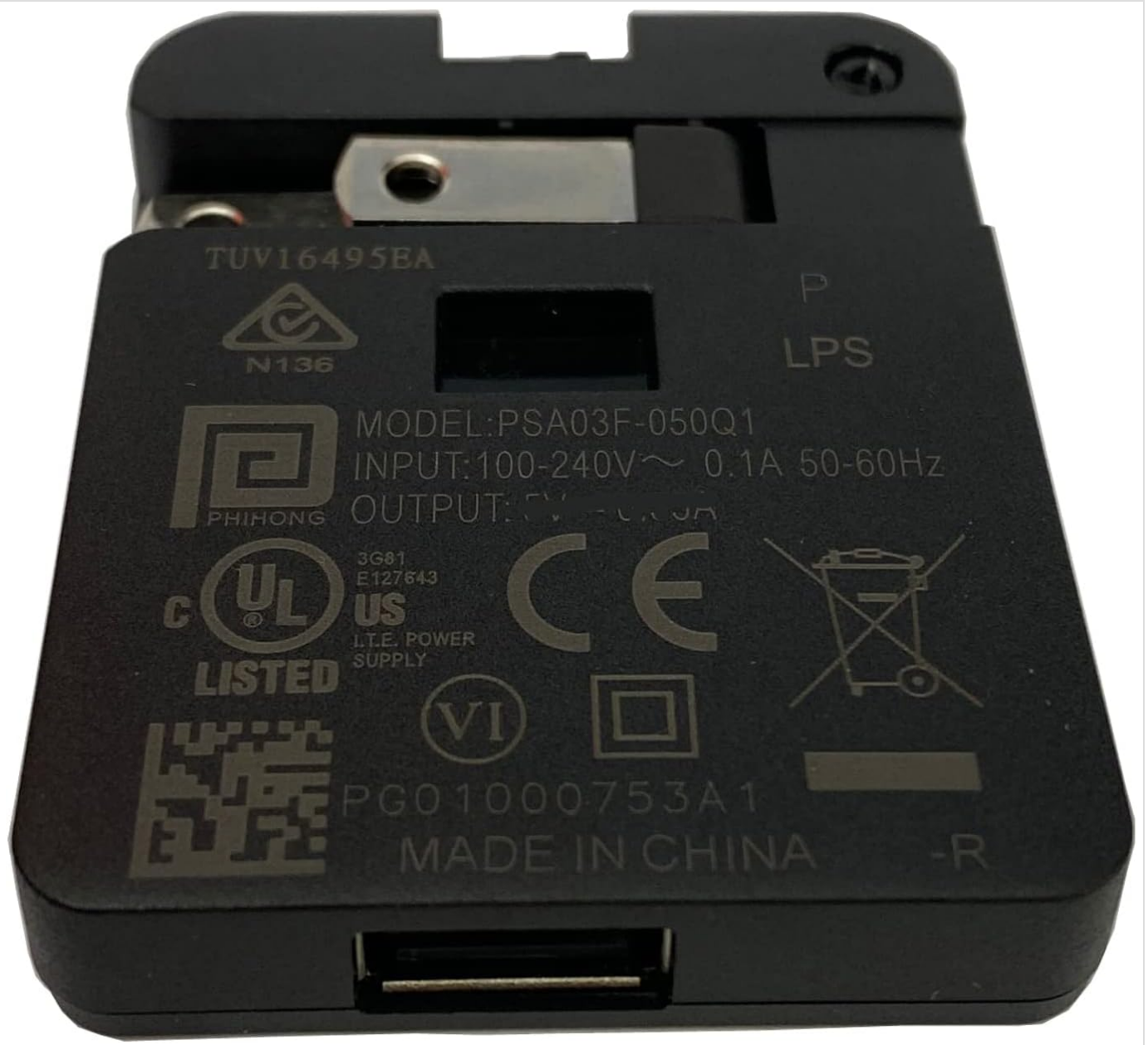
Image: A detailed close-up of the UpBright AC/DC adapter's label, showing input (100-240V) and output (5V) specifications, model number (PSA03F-050Q1), and various safety certifications (UL Listed, CE, etc.).
