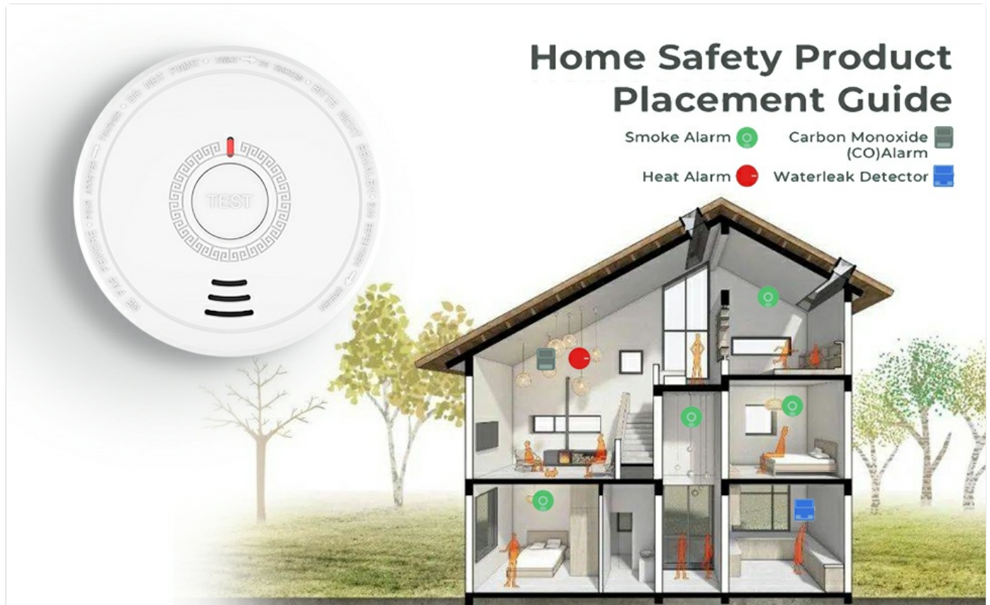
Image: A diagram illustrating recommended placement of smoke alarms (green circles) throughout a multi-story home for comprehensive safety coverage.
