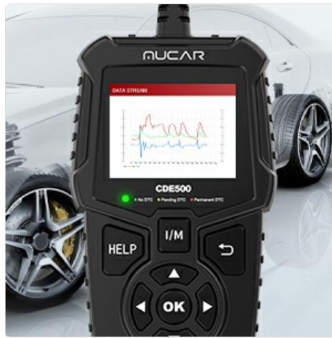
Image 3.4: The MUCAR CDE500 displaying a live data stream in a graphical format.
