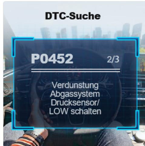
Image 3.2: The DTC Search screen, showing a sample trouble code P0452 and its description.
