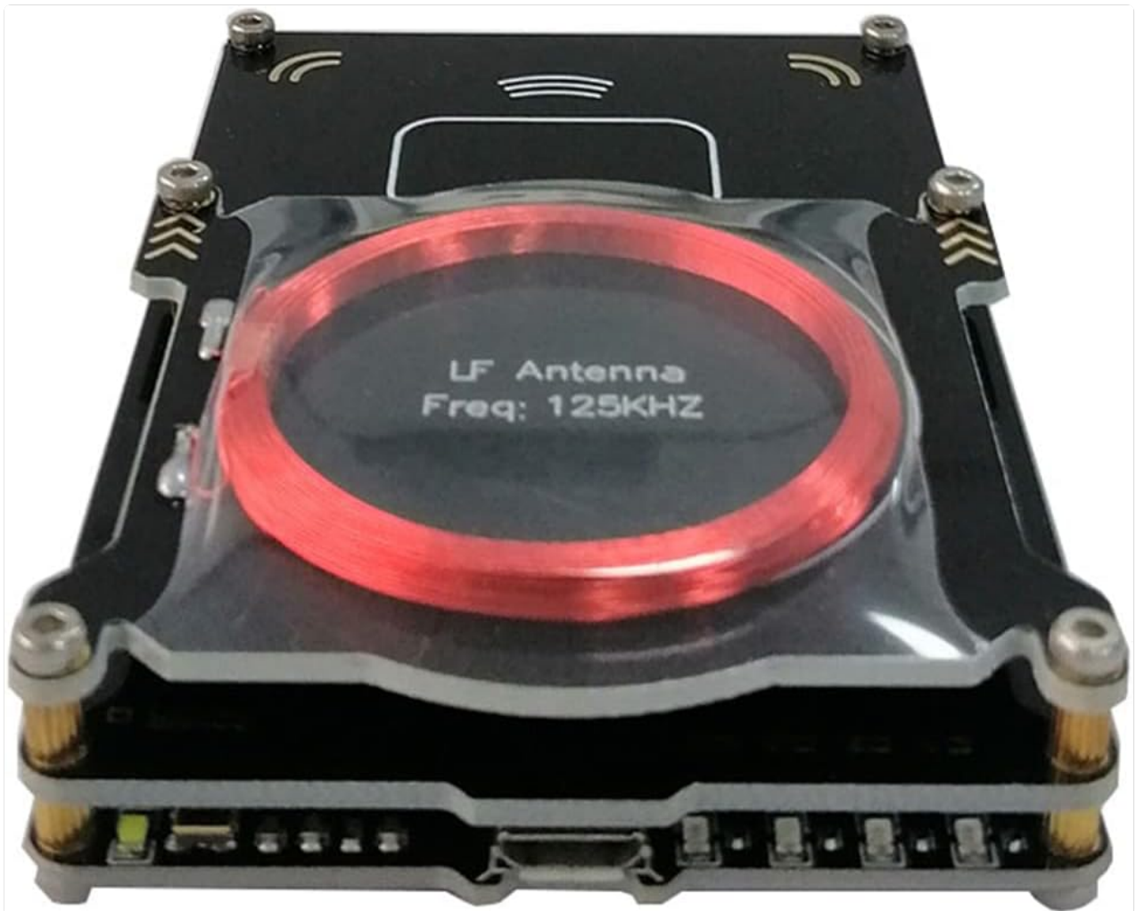
Image: A close-up view of the Proxmark3 Easy V3.0, highlighting the Low Frequency (LF) antenna area, which operates at 125KHz.
