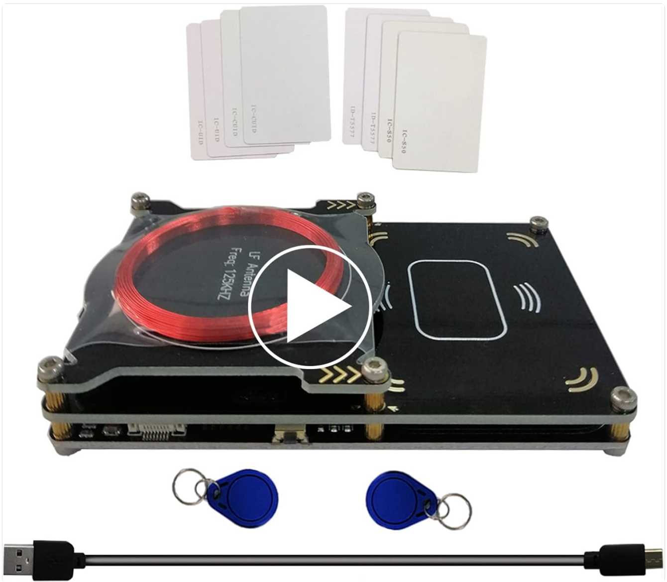
Image: The Proxmark3 Easy V3.0 device, accompanied by a USB data cable, several white RFID cards (IC-CUID, ID-T5577, IC-S50, IC-UID), and two blue RFID key tags.
